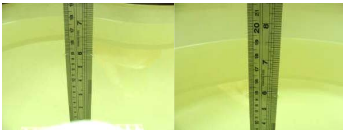
Photo of Liquid Height for Head SAR
