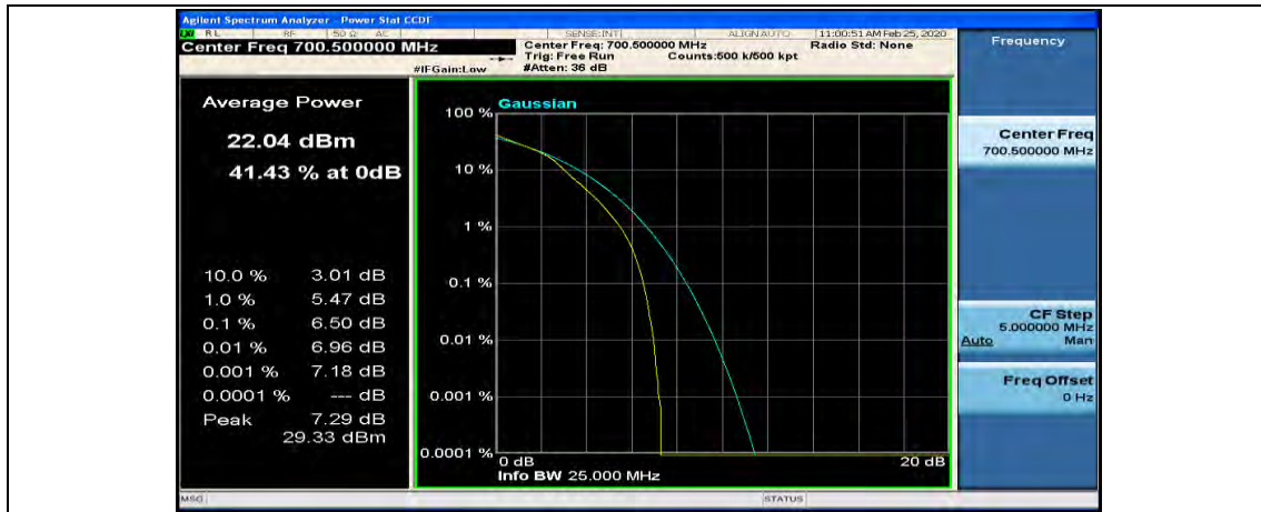
(Channel Bandwidth: 3 MHz)_MCH_16QAM_1RB#0
