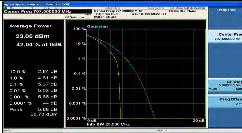
(Channel Bandwidth: 5 MHz)_MCH_QPSK_12RB#6
