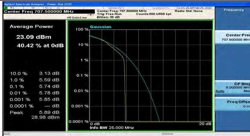
(Channel Bandwidth: 3 MHz)_MCH_16QAM_8RB#0
