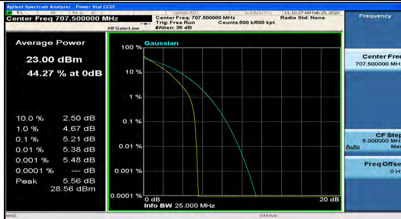
Channel Bandwidth: 10 MHz_MCH_QPSK_50RB#0
