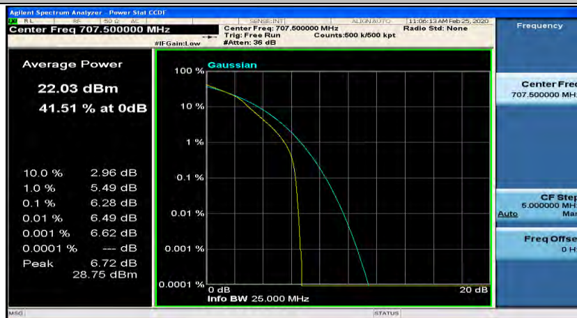
(Channel Bandwidth: 5 MHz)_MCH_16QAM_12RB#6
