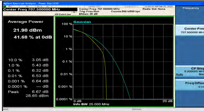
(Channel Bandwidth: 3 MHz)_MCH_16QAM_15RB#0
