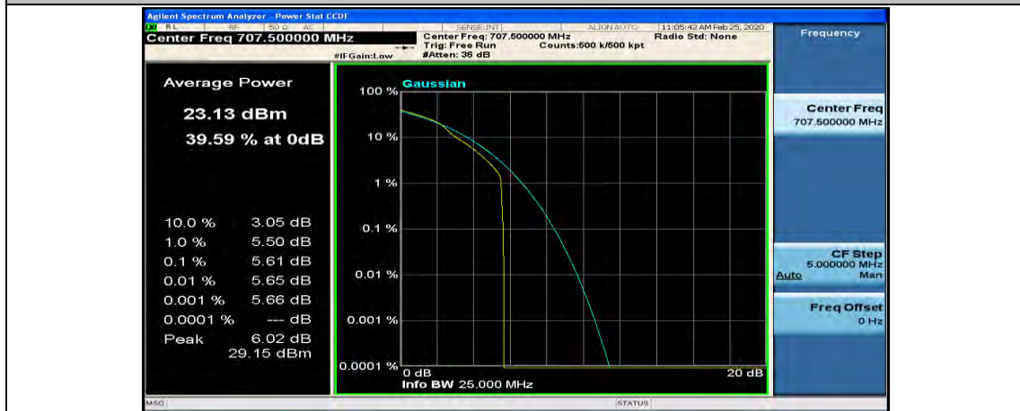
(Channel Bandwidth: 5 MHz)_MCH_16QAM_1RB#24
