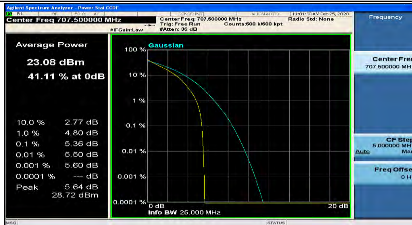
(Channel Bandwidth: 3 MHz)_MCH_QPSK_8RB#7
