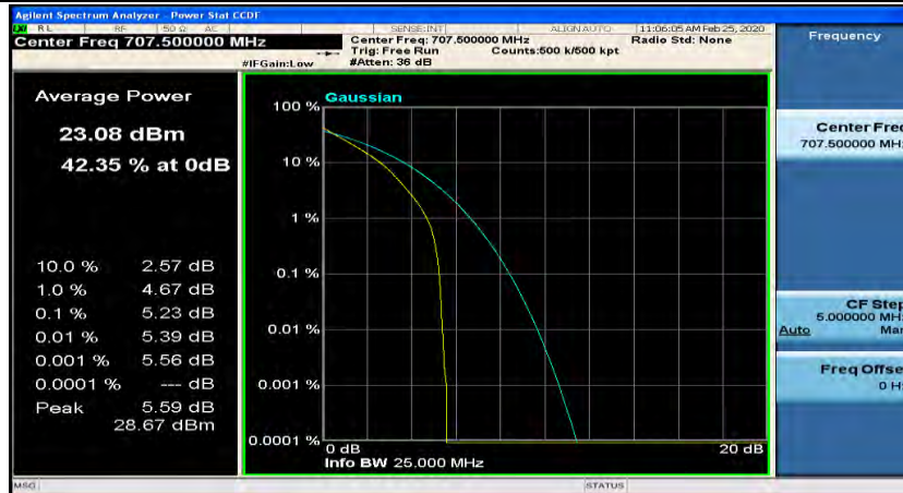
(Channel Bandwidth: 5 MHz)_MCH_QPSK_25RB#0
