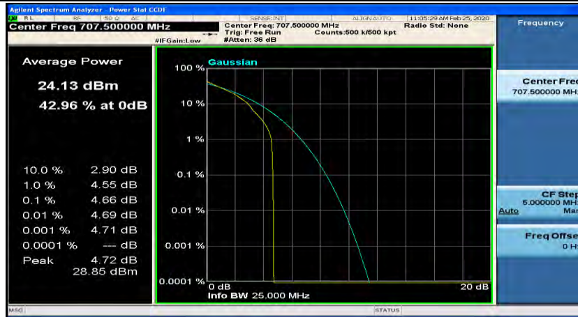
(Channel Bandwidth: 5 MHz)_MCH_QPSK_12RB#0
