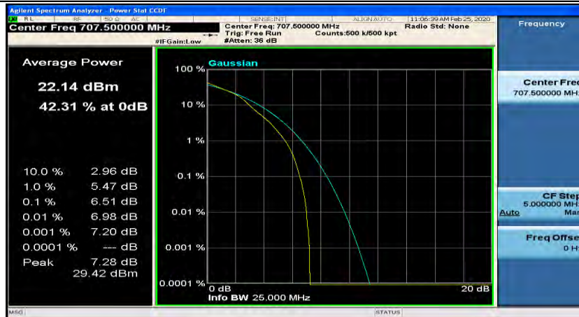
(Channel Bandwidth: 5 MHz)_MCH_16QAM_25RB#0
