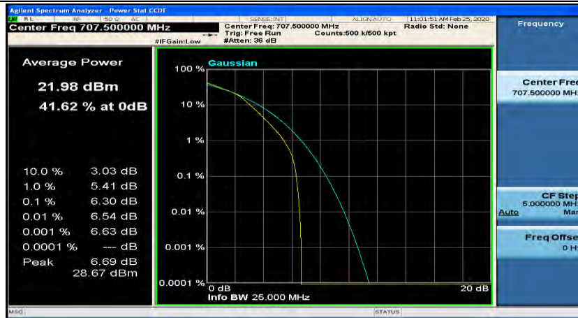
(Channel Bandwidth: 3 MHz)_MCH_16QAM_8RB#4
