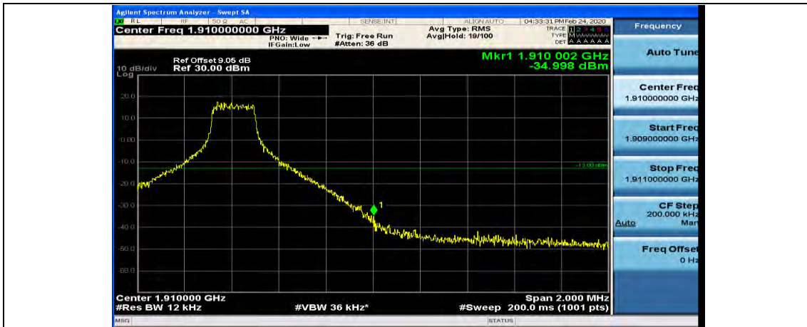
Channel Bandwidth: 10 MHz_HCH_QPSK_25RB#0
