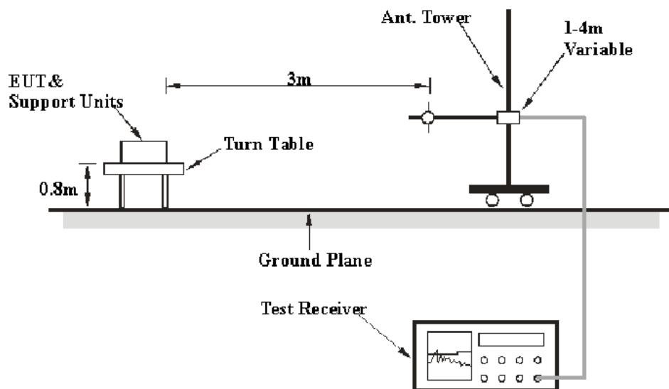
The radiated emission tests were performed in the 3 meters, using the setup accordance with the ANSI C63.10-2013. The specification used was the FCC Part 15.235(a) & 15.235 (b) &15.209 limits.
