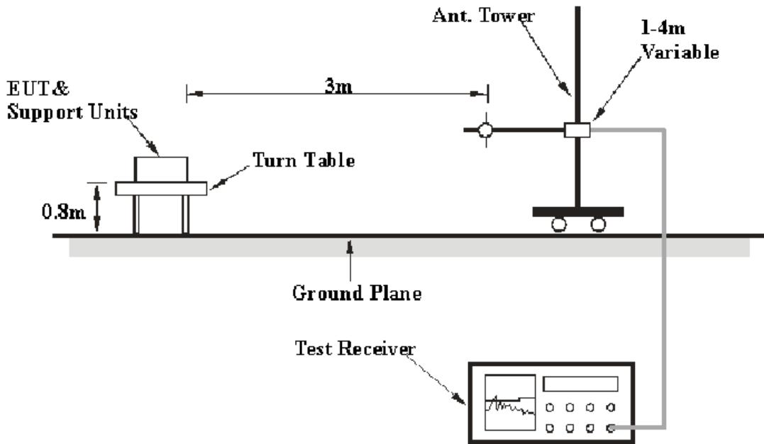
The radiated emission tests were performed in the 3 meters, using the setup accordance with the ANSI ANSI C63.10-2013. The specification used was the FCC Part 15.205 and 15.209 and 15.227 limits.
