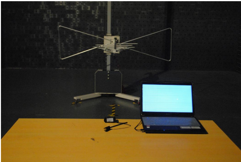
Radiated Emission test view
