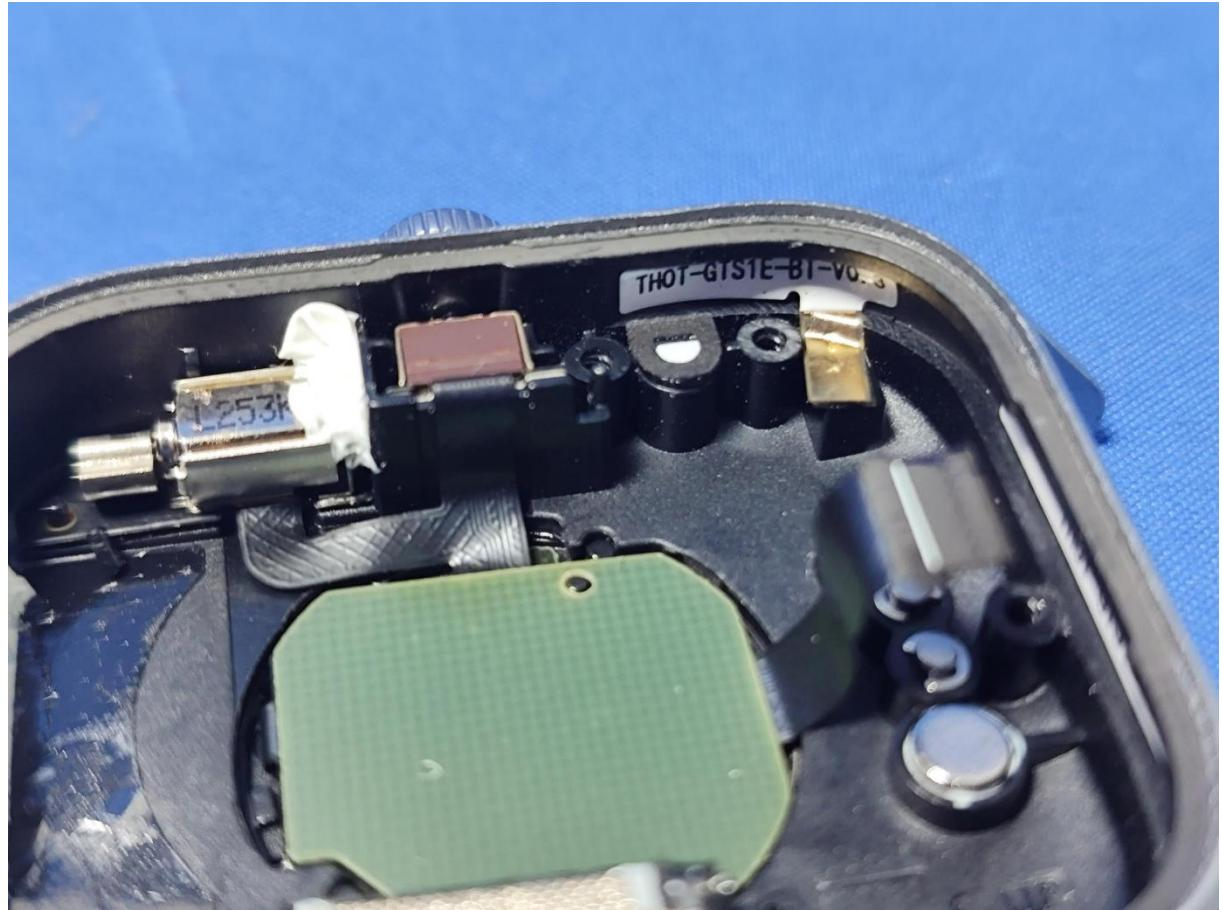
A photograph showing the internal components of the smartwatch. The watch is open, revealing a green rectangular antenna board. Other internal parts like a red component, a blue button, and a metal connector are visible. A small white label with the text "THOT-GTS1E-BT-V0.1" is visible on the top right. The watch is set against a blue background. |
