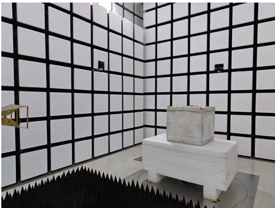
Radiated Emission Above 1GHz View
