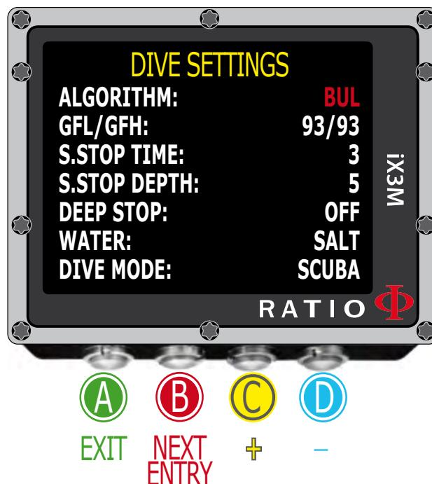
**S. STOP TIME:** It sets the Safety Stop's time in minutes. You can set the time from 0 to 9 minutes (if 0 the Safety Stop is omitted)
