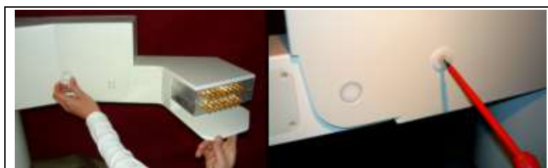
Figure 13: Bring the arm to the horizontal position and apply one insert to the inner hole and one to the outer hole.
