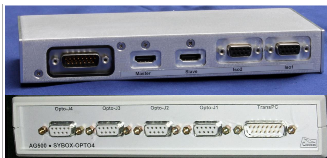
Figure 6: Sybox front side – Sybox 2 (top) and Sybox-Opto4 (bottom)
