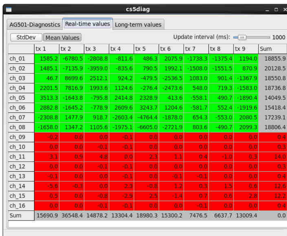
Figure 7: Real-time mean values - the low total values of channel 9 to 16 indicate incorrect values for these channels (defective or missing sensors)
