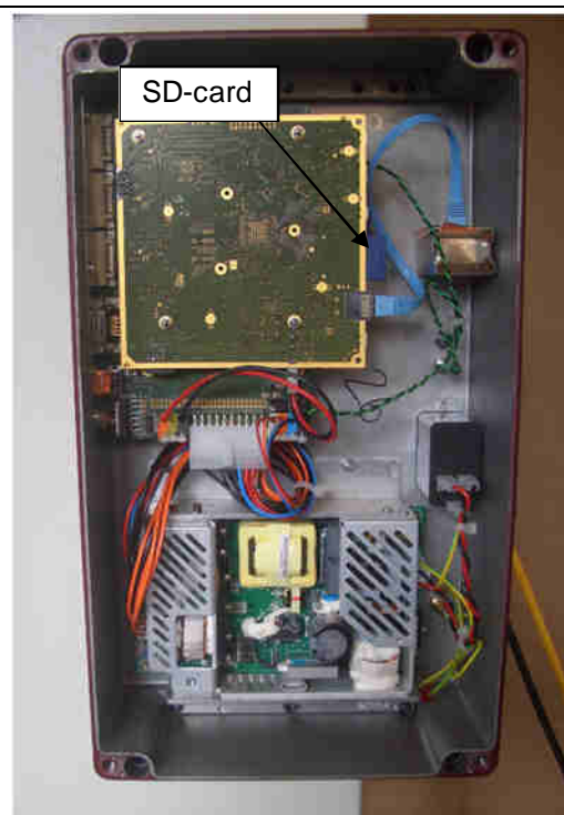
Figure 2: The SD-card is mounted to the Z2-FPGA
