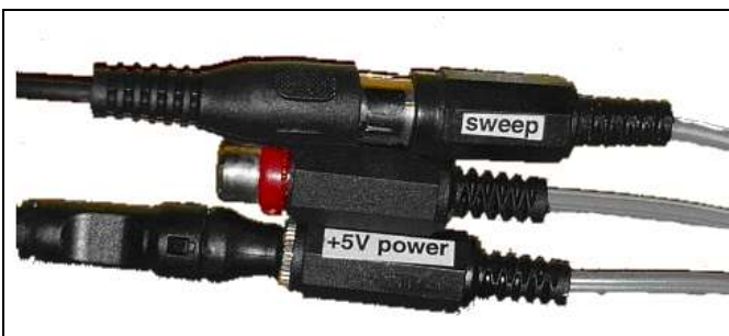
Figure 11: Power supply connection for Sybox-Opto4
