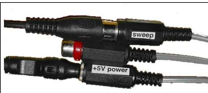
Figure 43: Power supply connection for Sybox-Opto4
