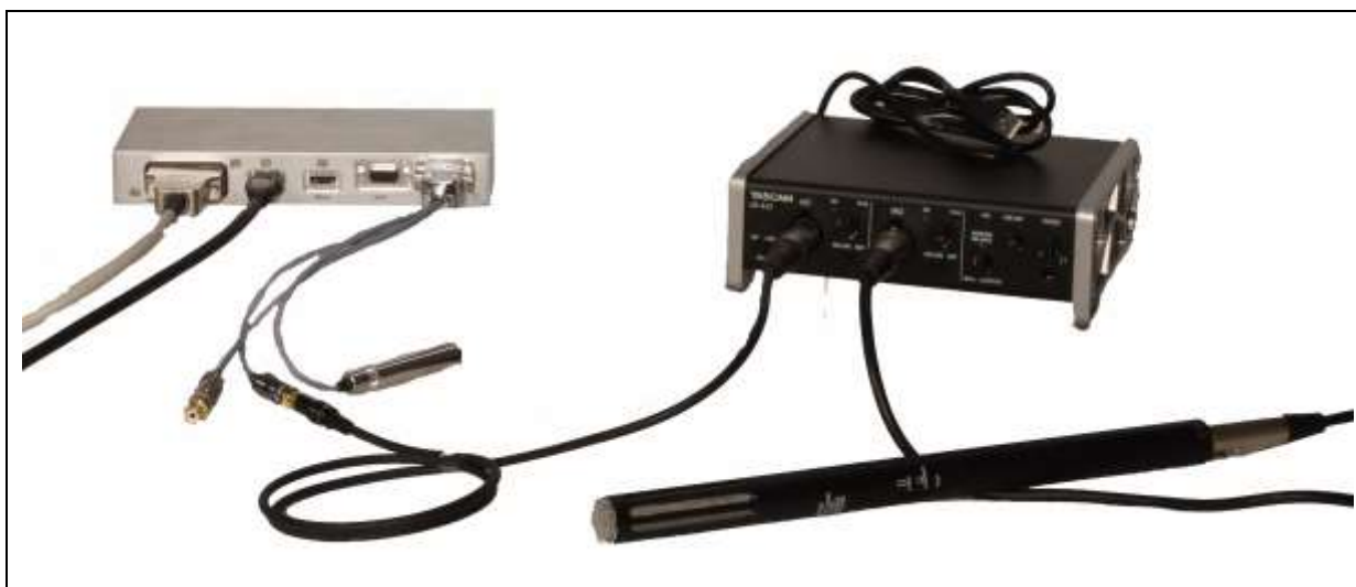
Figure 32: The Wiring of Tascam US-2x2 sound card with the Sybox2
