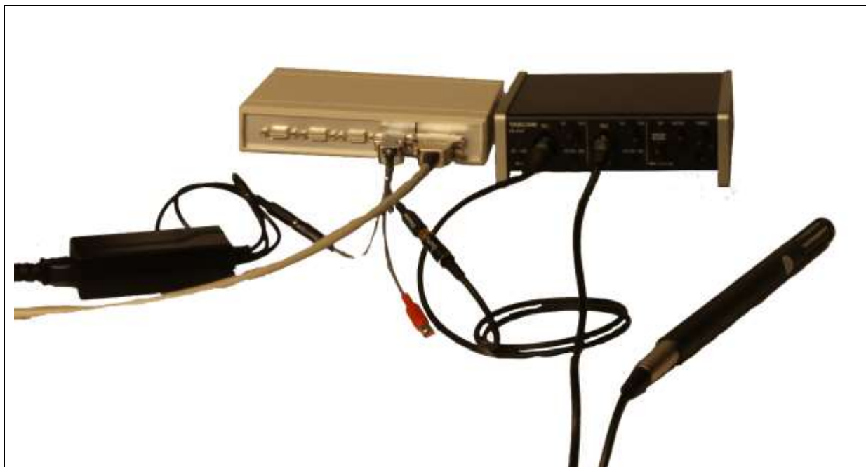
Figure 44: The Wiring of Tascam US-2x2 sound card with the Sybox-Opto4
