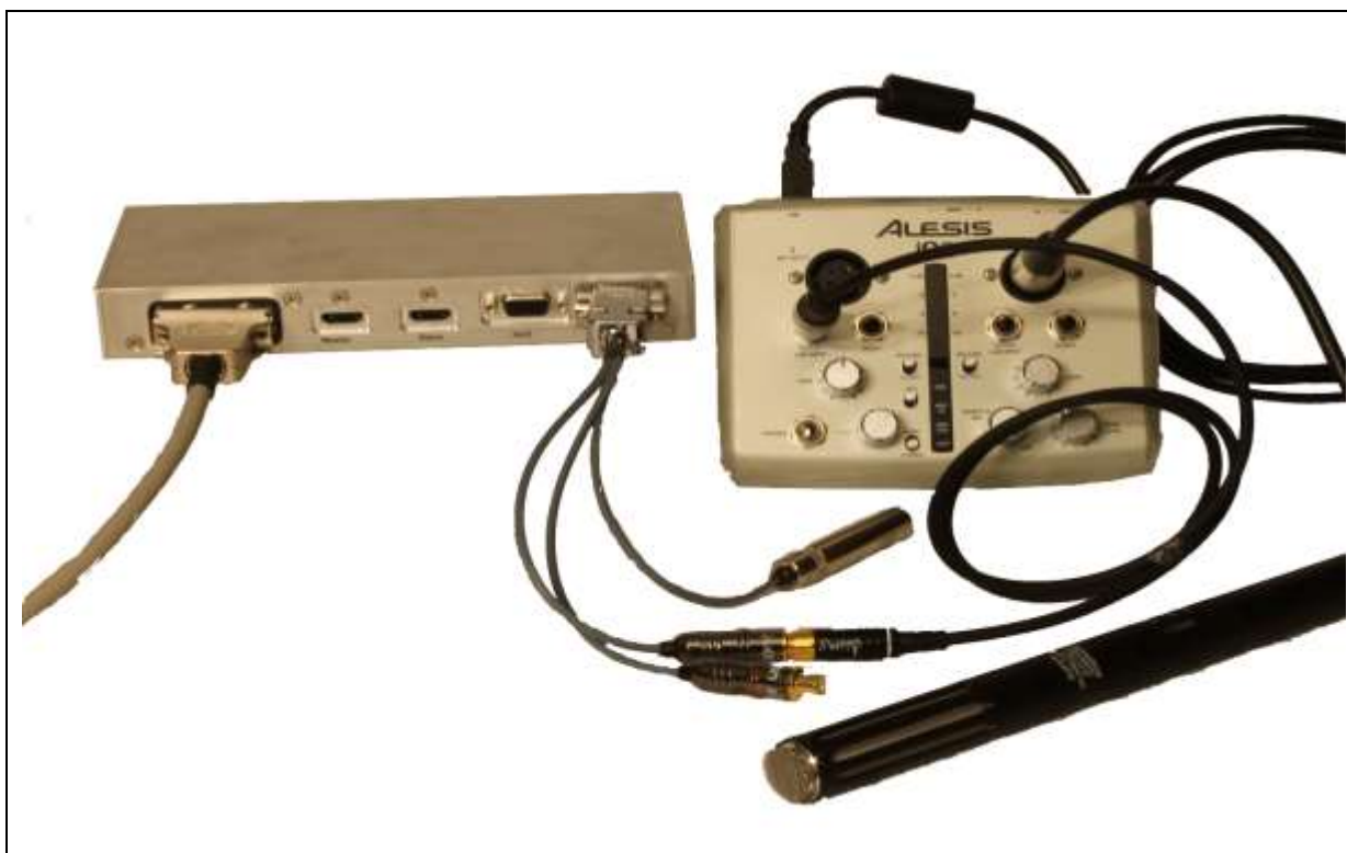
Figure 22: The Wiring of Alesis sound card with the Sybox 2
