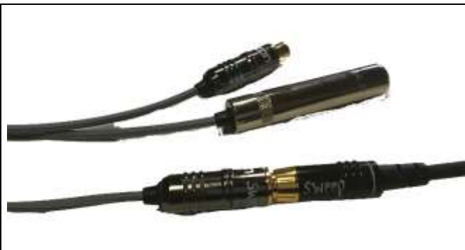
Figure 31: sweep - adapter connection
