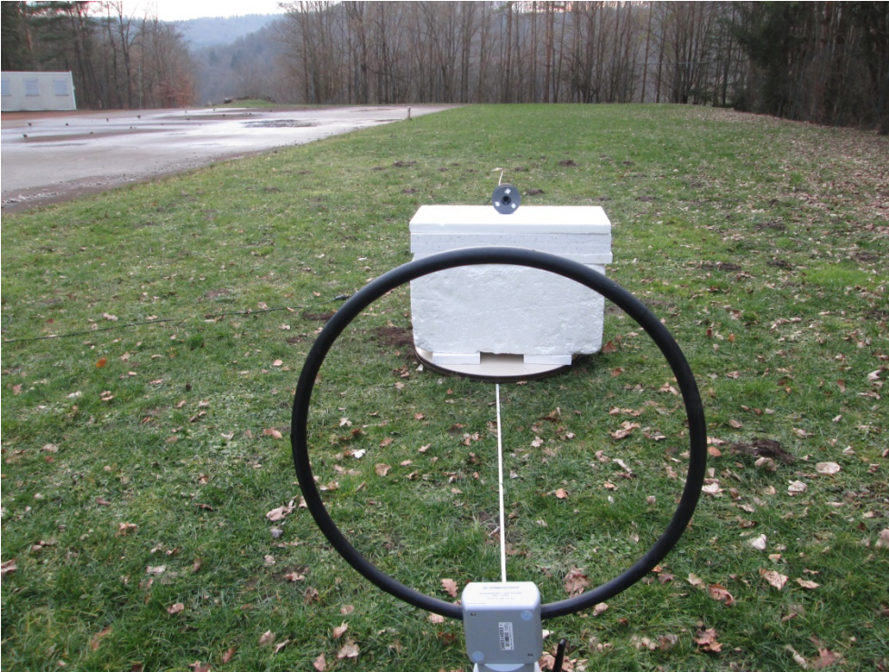
Photo A1-3: Radiated emissions measurement at 3 m distance, 9 kHz – 30 MHz, reference measurement at open field site
