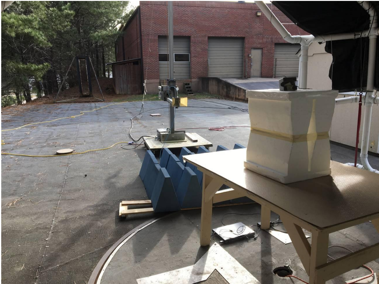
Figure 6. Radiated Emissions Testing (Above 1 GHz)
