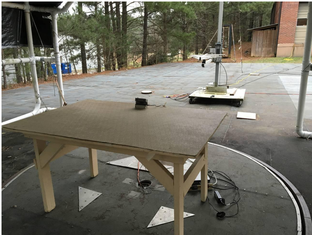
Figure 5. Radiated Emissions Testing (200 MHz-1000 MHz)
