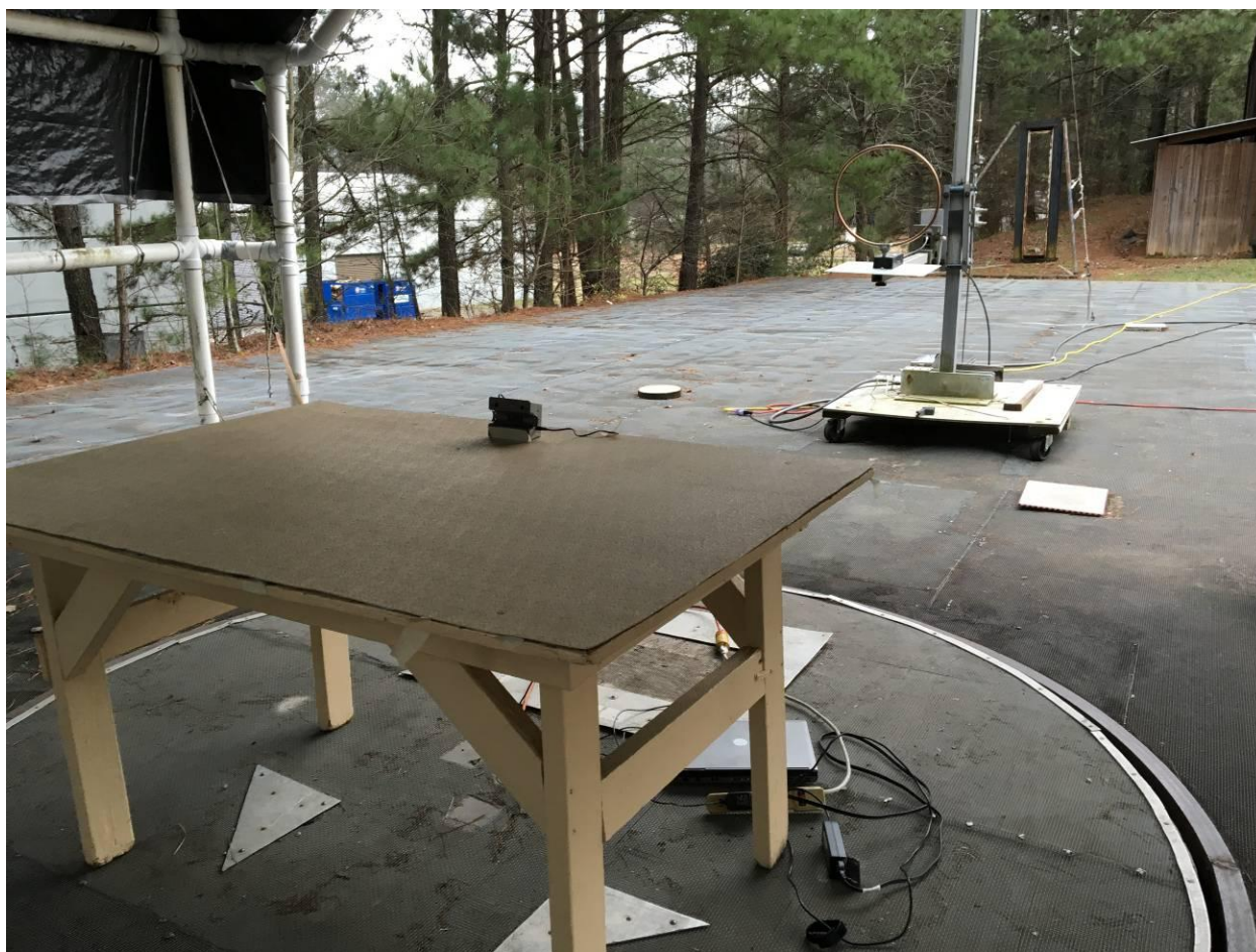
Figure 3. Radiated Emissions Testing (Below 30 MHz)
