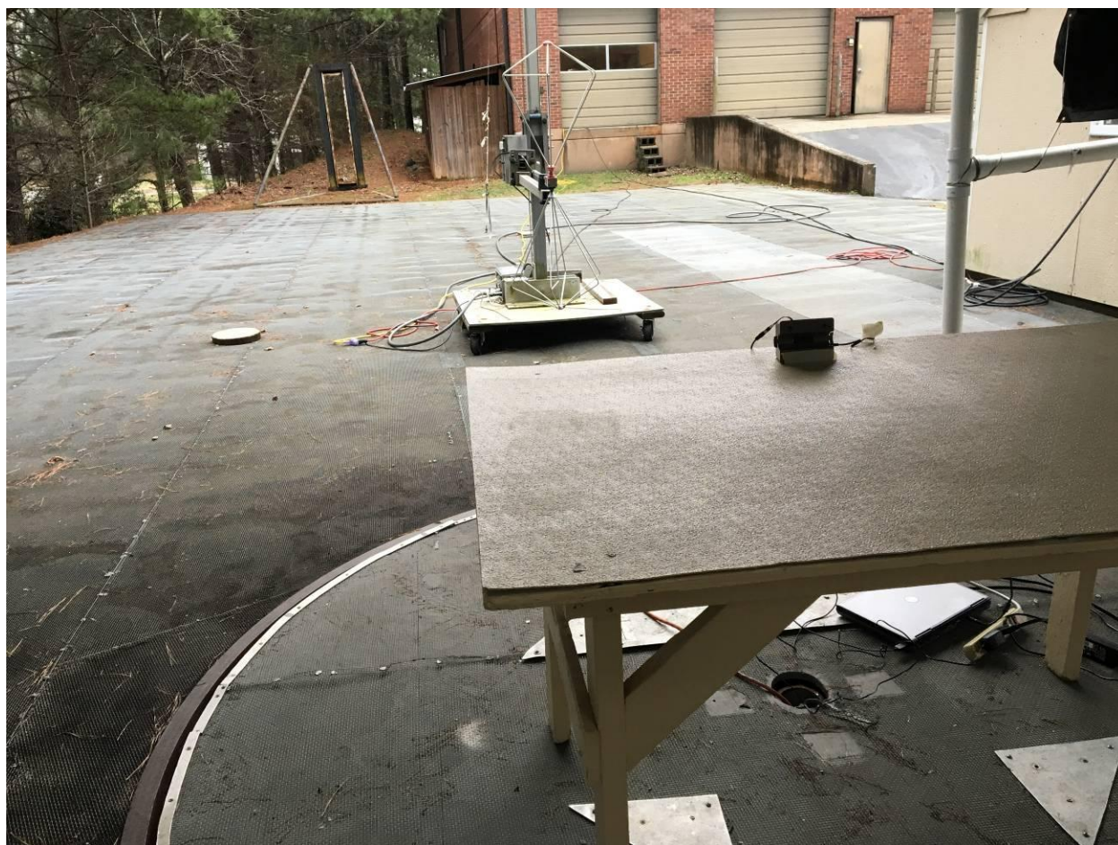
Figure 4. Radiated Emissions Testing (30 MHz-200 MHz)
