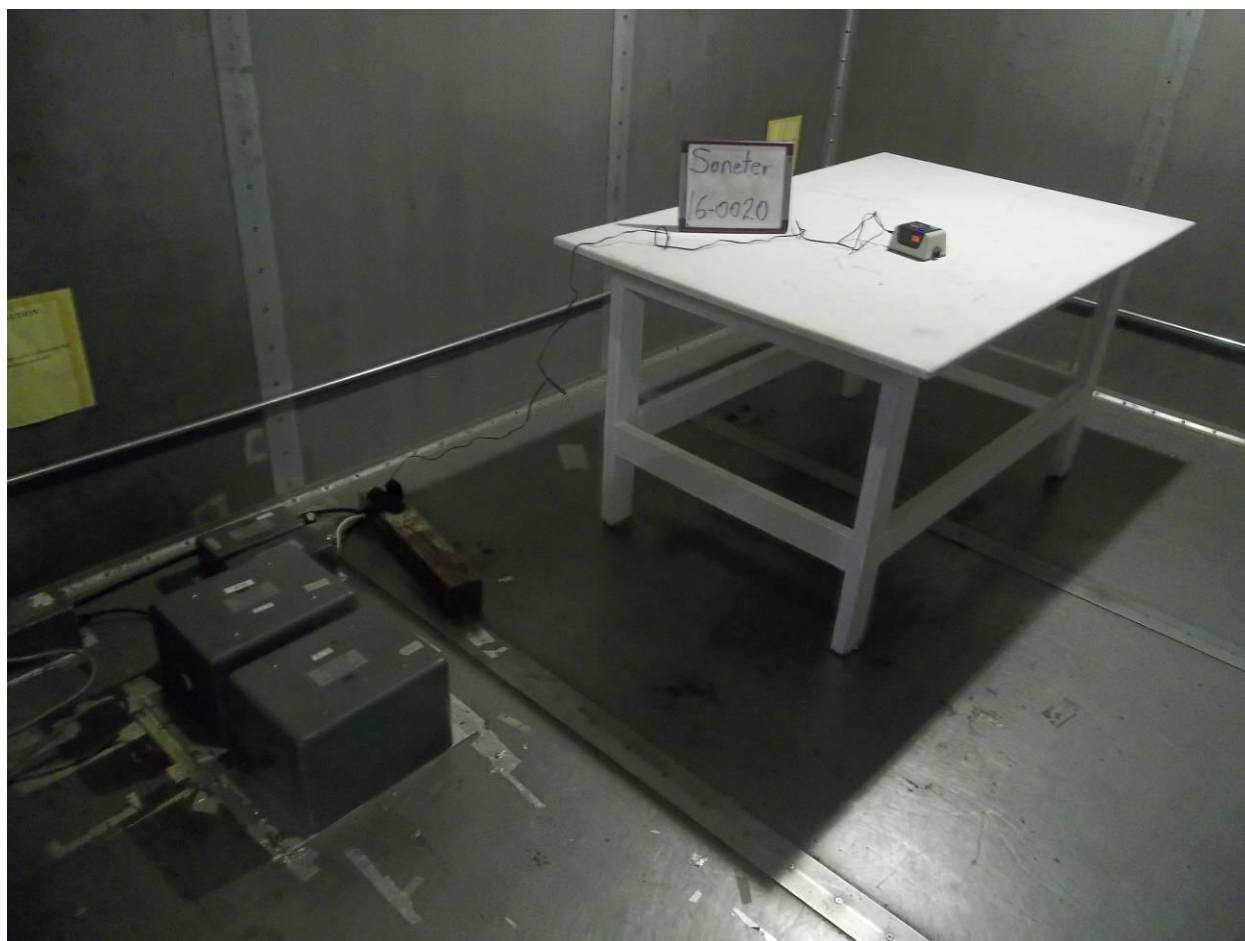
Figure 7. Power Line Conducted Emissions Test Configuration
