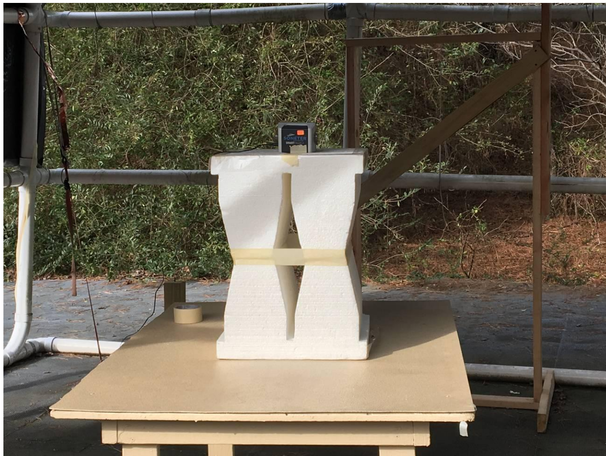
Figure 2. Radiated Emissions Test configuration Above 1 GHz
