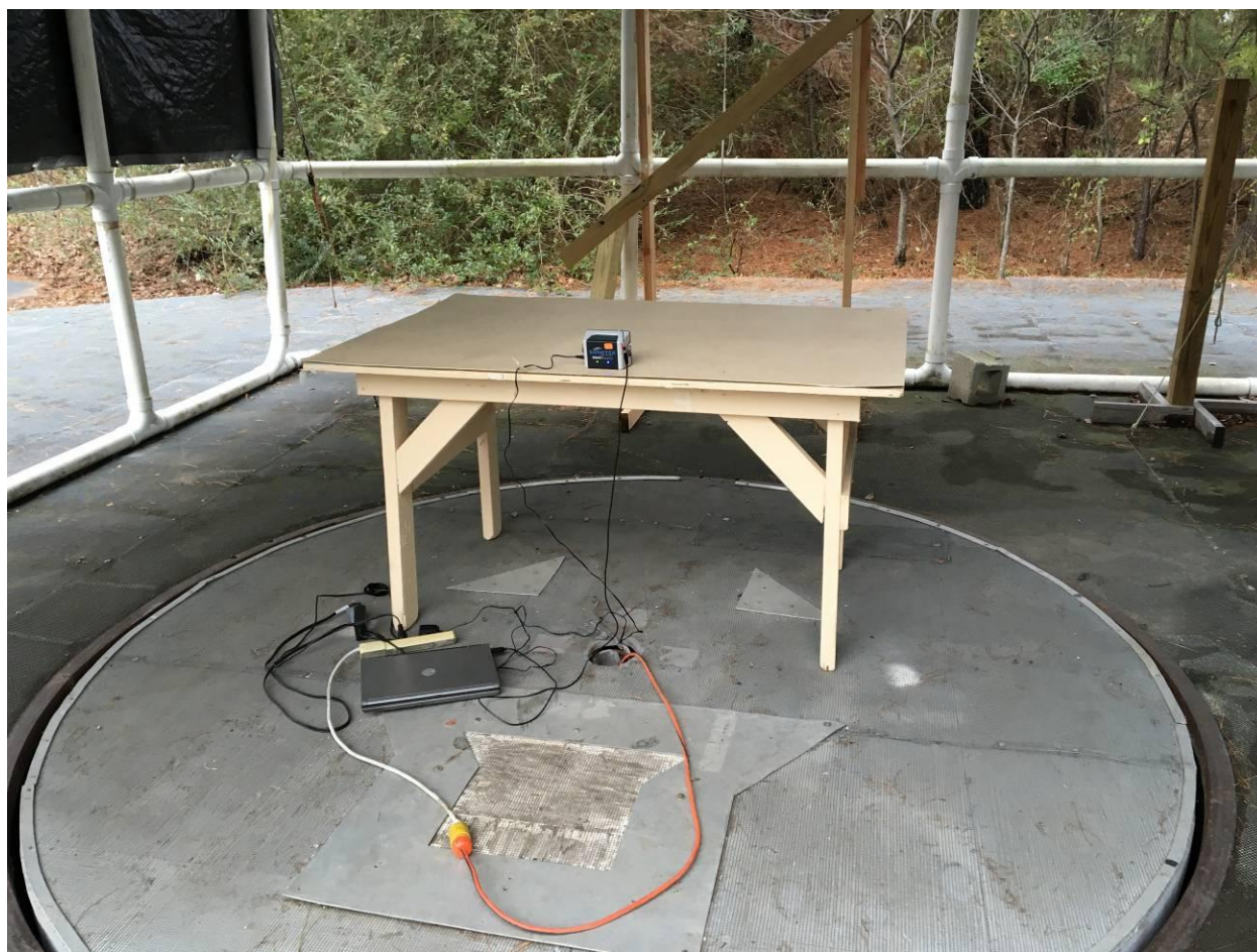
Figure 1. Radiated Emissions Test Configuration Below 1 GHz
