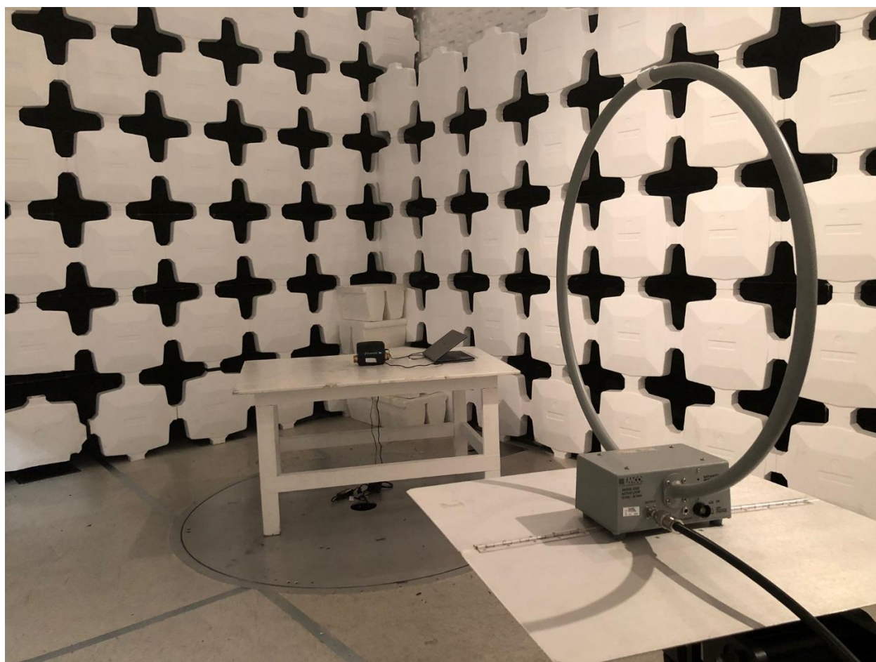
Figure 1. Radiated Emissions Test Configuration (Below 30 MHz)
