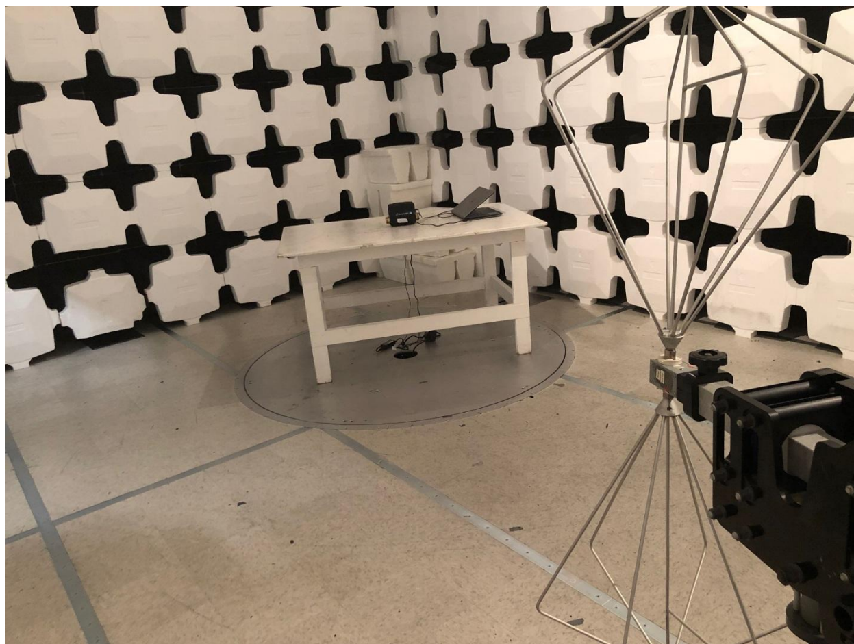
Figure 2. Radiated Emissions Test Configuration (30-200 MHz)
