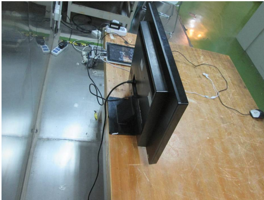
Conducted Emissions - Side View (HDMI Mode)
