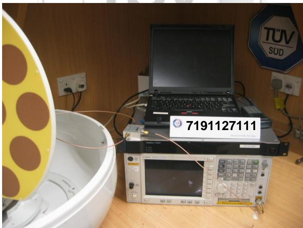
**Unwanted Emissions at Antenna Terminal Test Setup**
