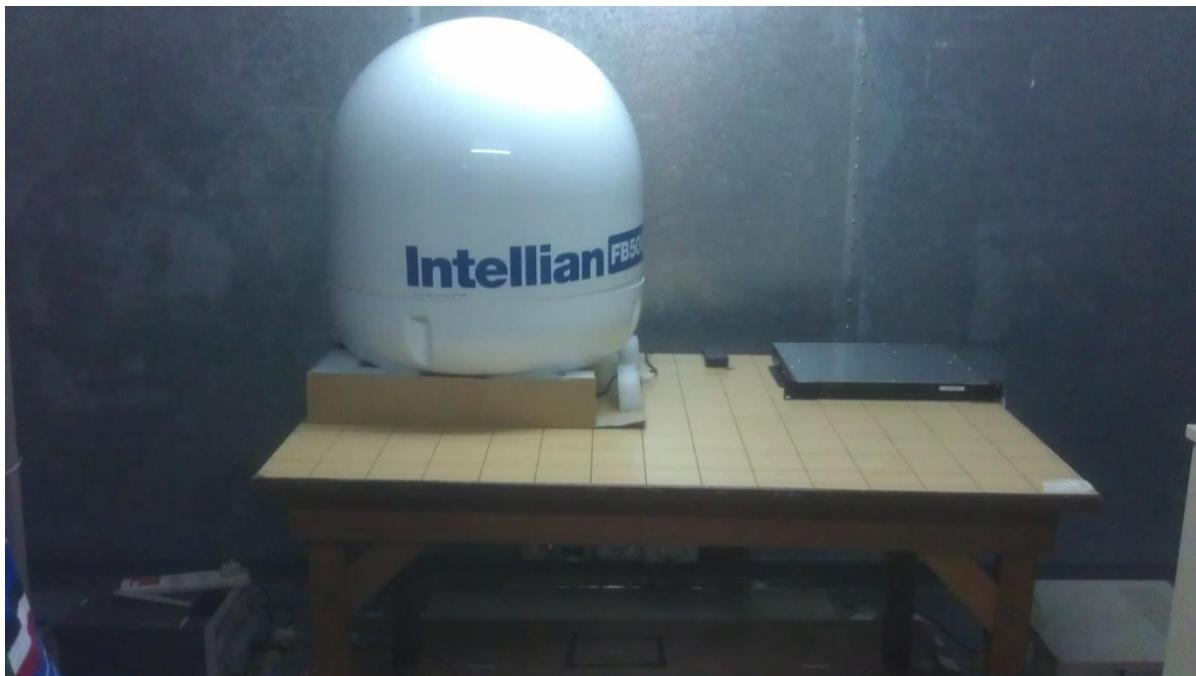
Conducted Emissions Test Setup (Front View)
