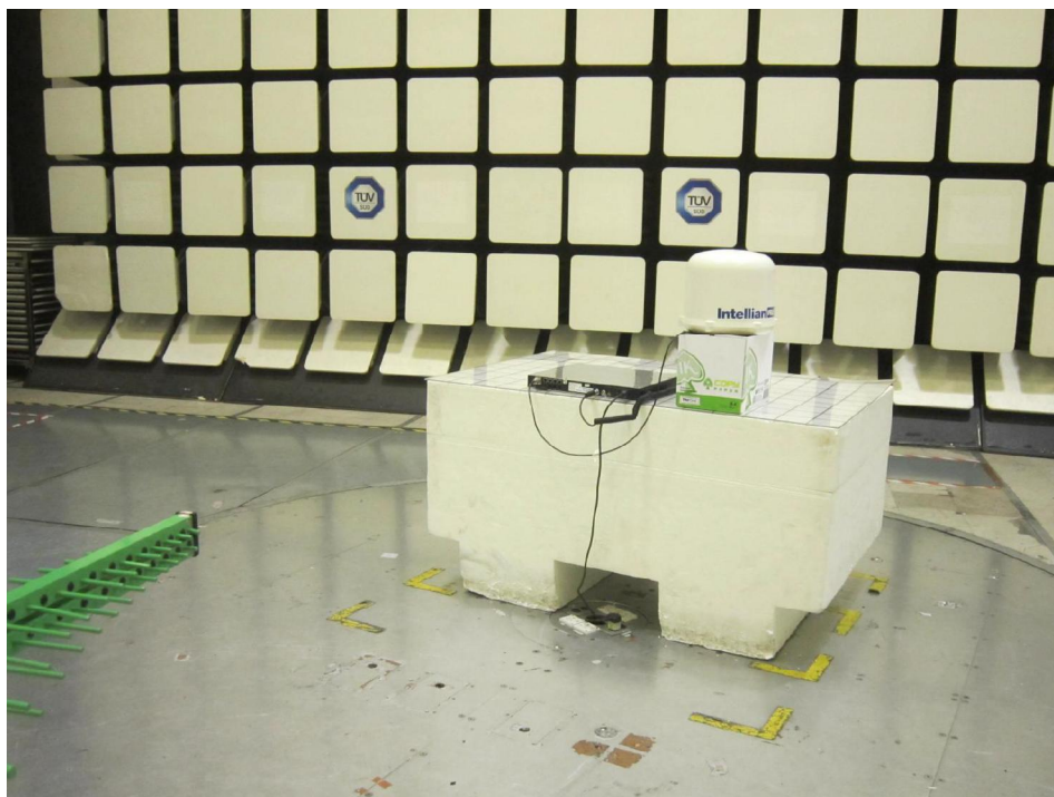
Radiated Emissions Test Setup (Front View)
