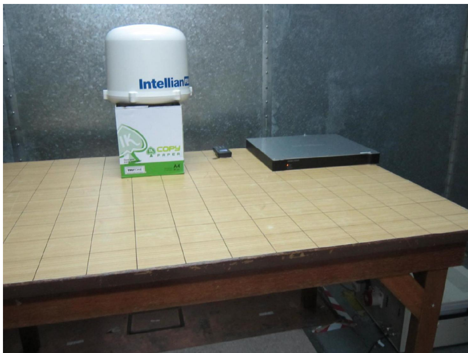
Conducted Emissions Test Setup (Front View)
