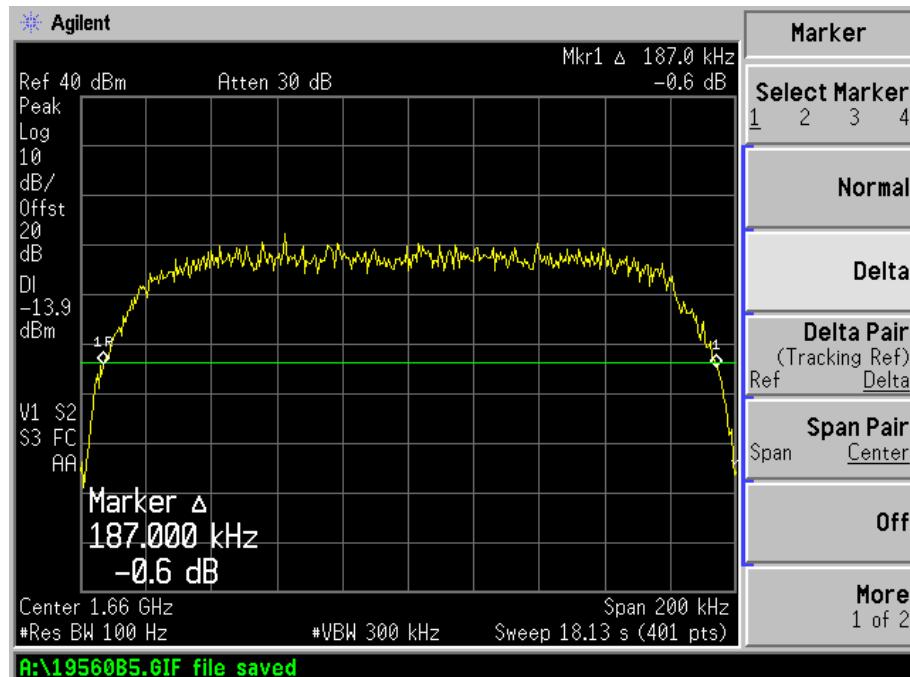
UNWANTED EMISSIONS AT ANTENNA TERMINAL TEST
