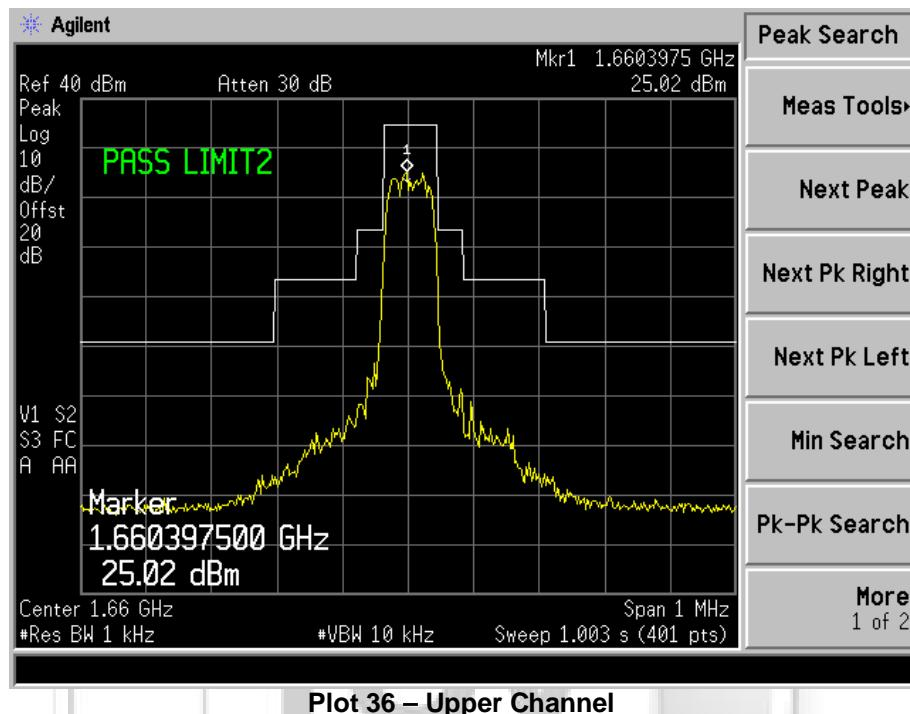
**UNWANTED EMISSIONS AT ANTENNA TERMINAL TEST**
