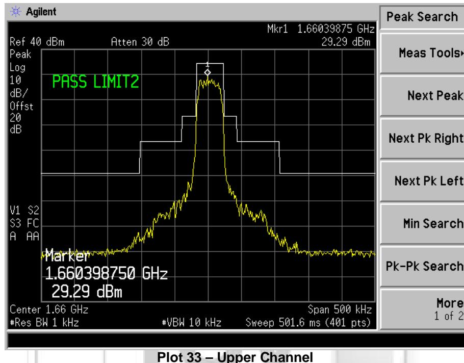
UNWANTED EMISSIONS AT ANTENNA TERMINAL TEST
