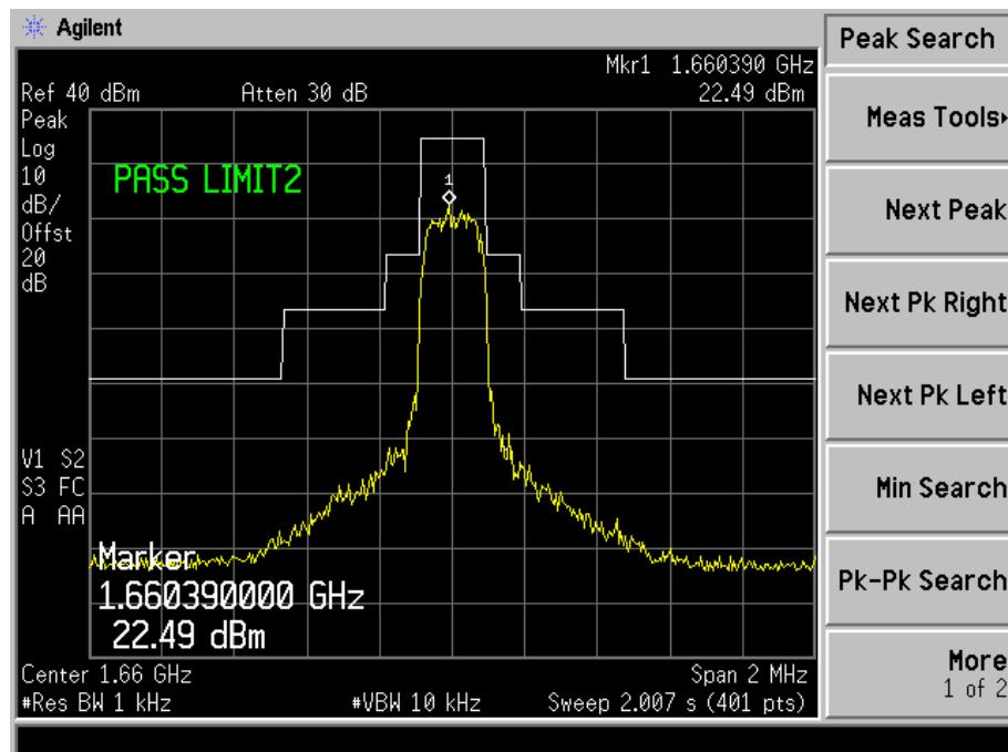
**UNWANTED EMISSIONS AT ANTENNA TERMINAL TEST**
