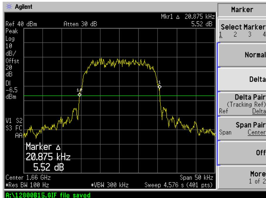
UNWANTED EMISSIONS AT ANTENNA TERMINAL TEST
