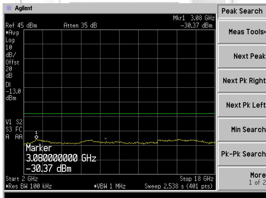
**UNWANTED EMISSIONS AT ANTENNA TERMINAL TEST**
