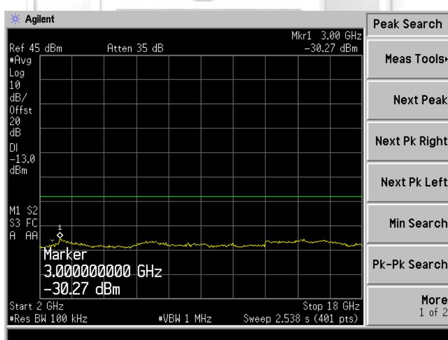
**UNWANTED EMISSIONS AT ANTENNA TERMINAL TEST**
