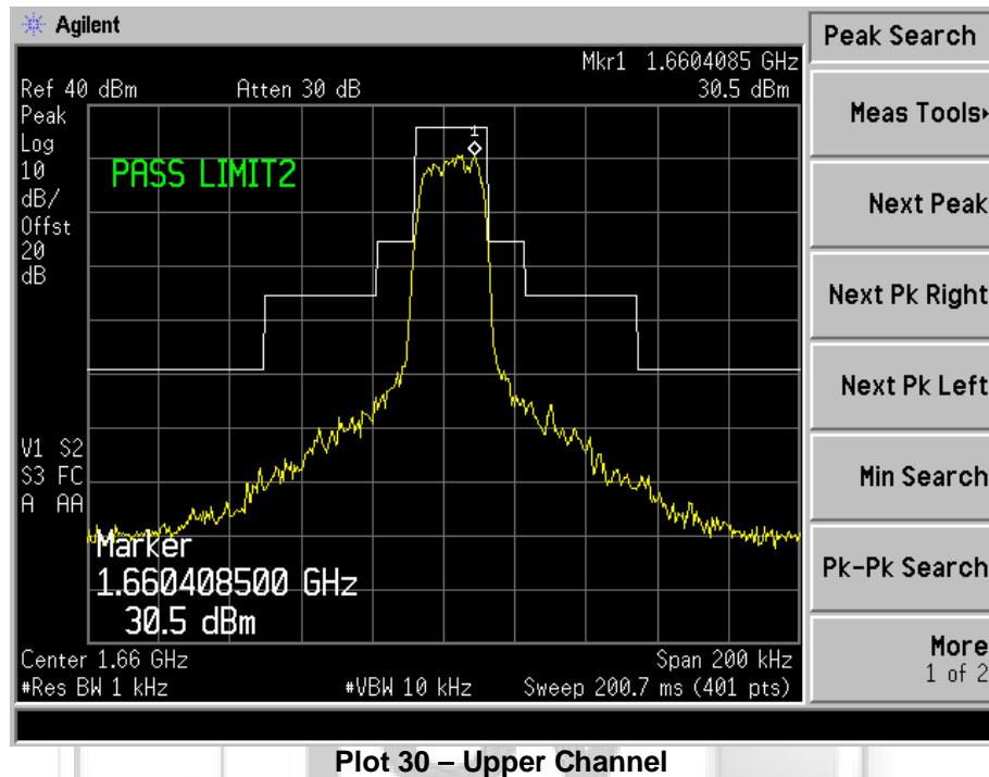
**UNWANTED EMISSIONS AT ANTENNA TERMINAL TEST**
