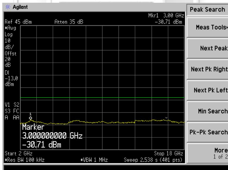
**UNWANTED EMISSIONS AT ANTENNA TERMINAL TEST**
