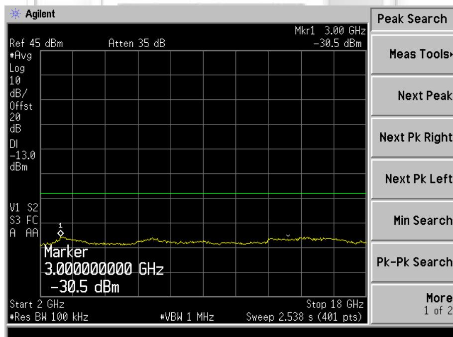
**UNWANTED EMISSIONS AT ANTENNA TERMINAL TEST**
