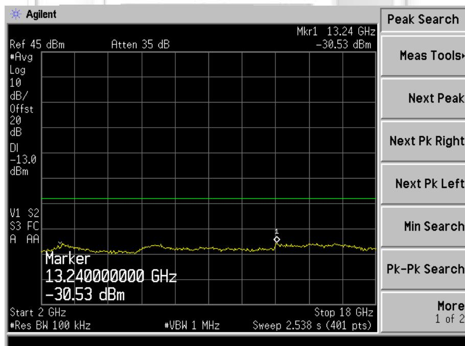
**UNWANTED EMISSIONS AT ANTENNA TERMINAL TEST**
