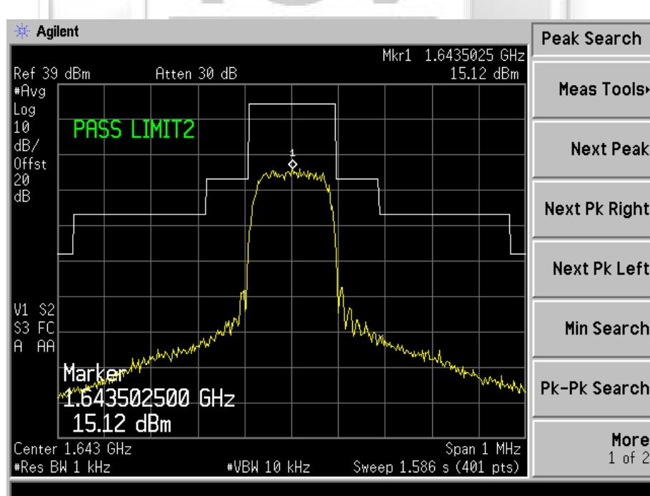
UNWANTED EMISSIONS AT ANTENNA TERMINAL TEST
