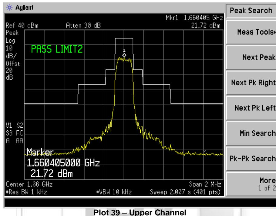
**UNWANTED EMISSIONS AT ANTENNA TERMINAL TEST**
