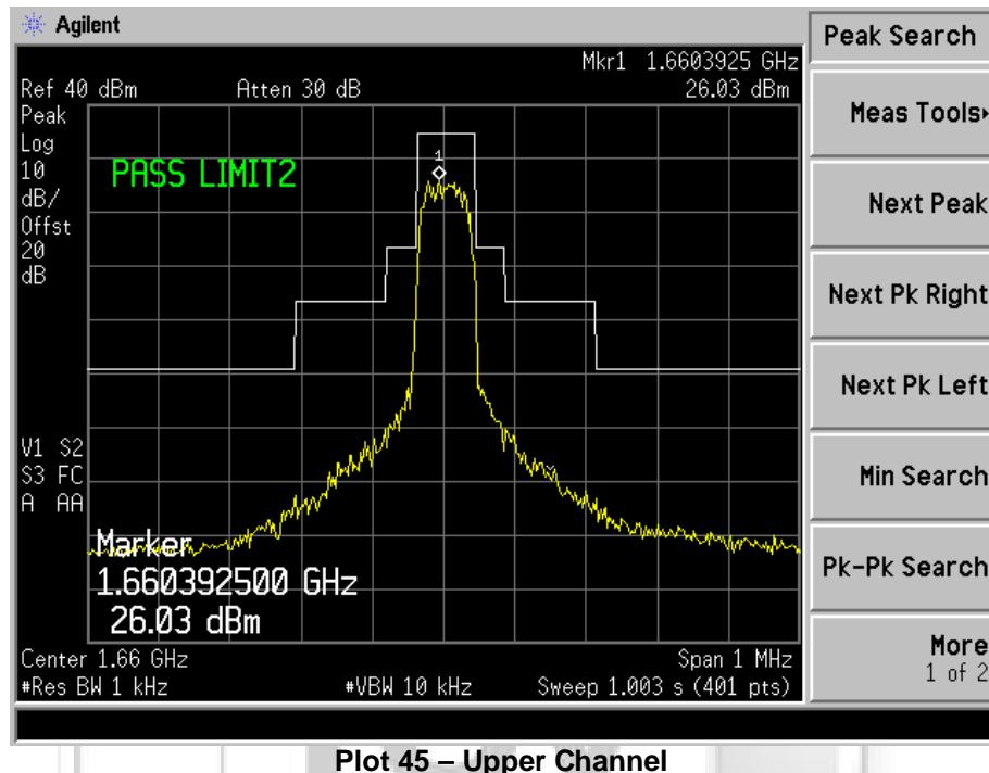
**UNWANTED EMISSIONS AT ANTENNA TERMINAL TEST**
