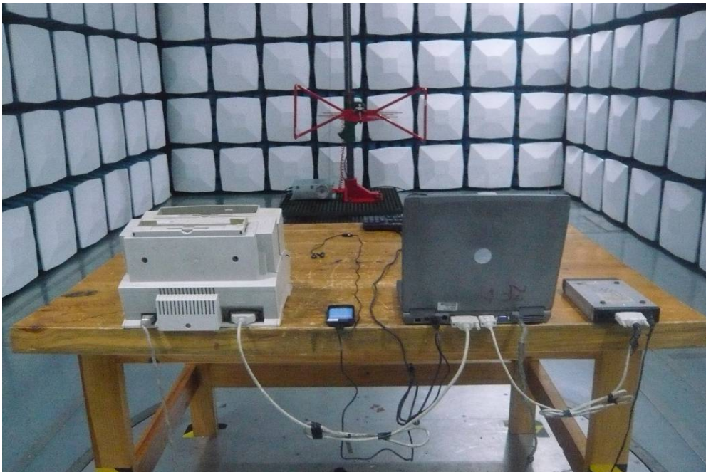
Radiated Emissions –Rear View (Below 1GHz)
