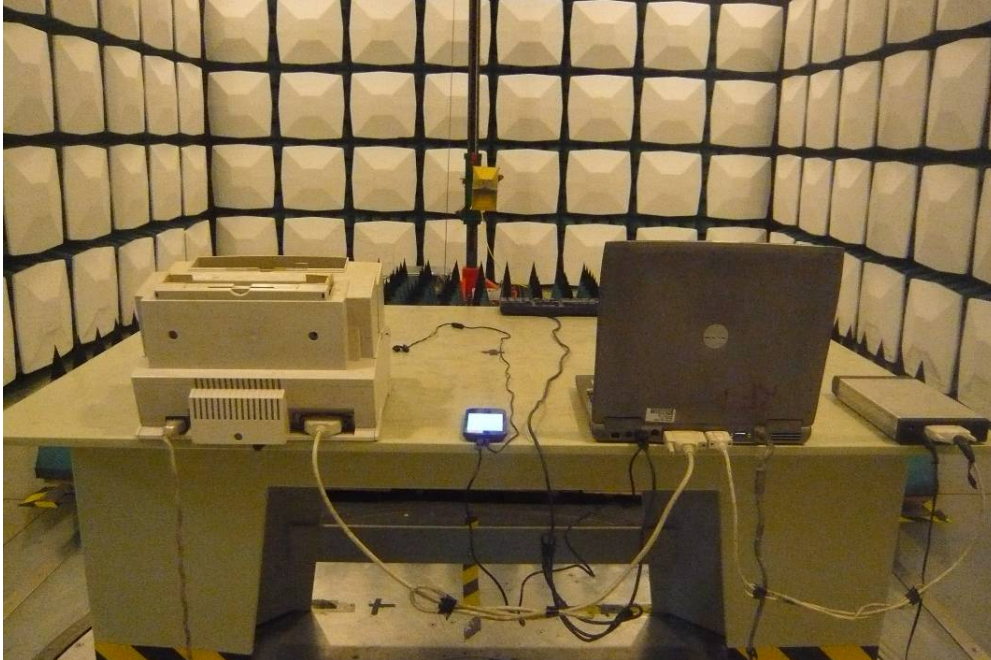
Radiated Emission –Rear View (Above 1 GHz)
