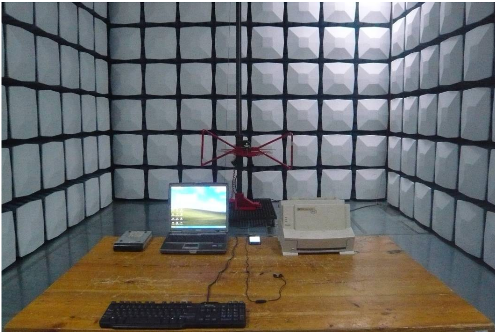
Radiated Emissions –Front View (Below 1GHz)
