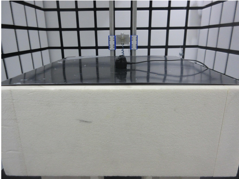
Radiated Emission Test below 1GHz
