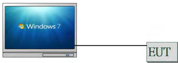
Fig. 2-2 Conducted (Antenna Port) Emission Configuration
