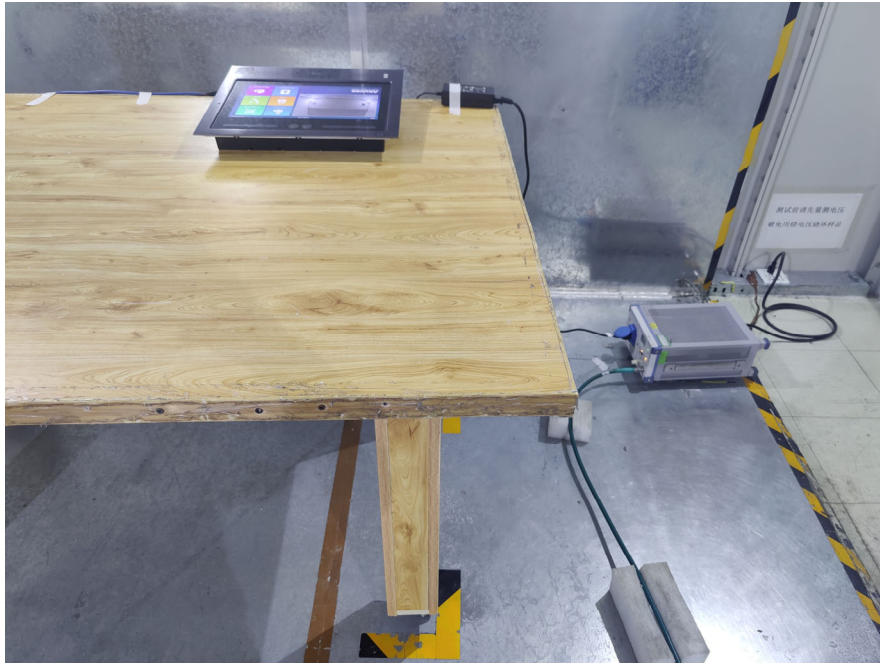
Conducted Emissions (Side View)
