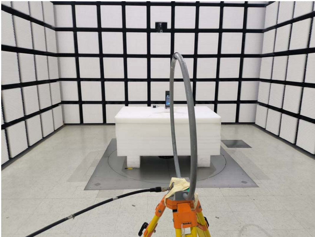
Radiated Emission Below 1GHz View Ground-parallel
