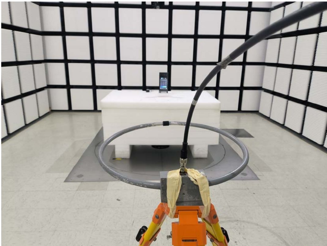
Radiated Emission Below 1GHz View Ground-parallel
