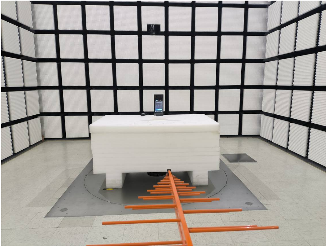
Radiated Emission Below 1GHz View-Powered byPoE
