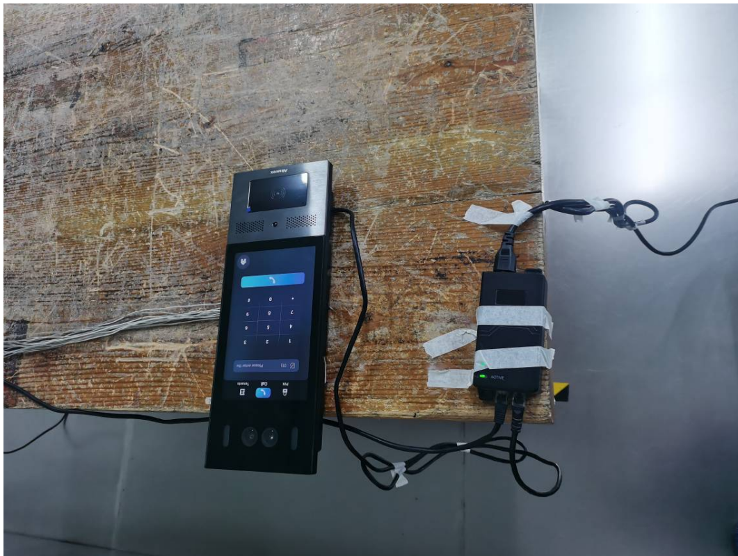
Conducted Emissions Side View-Powered byPoE
