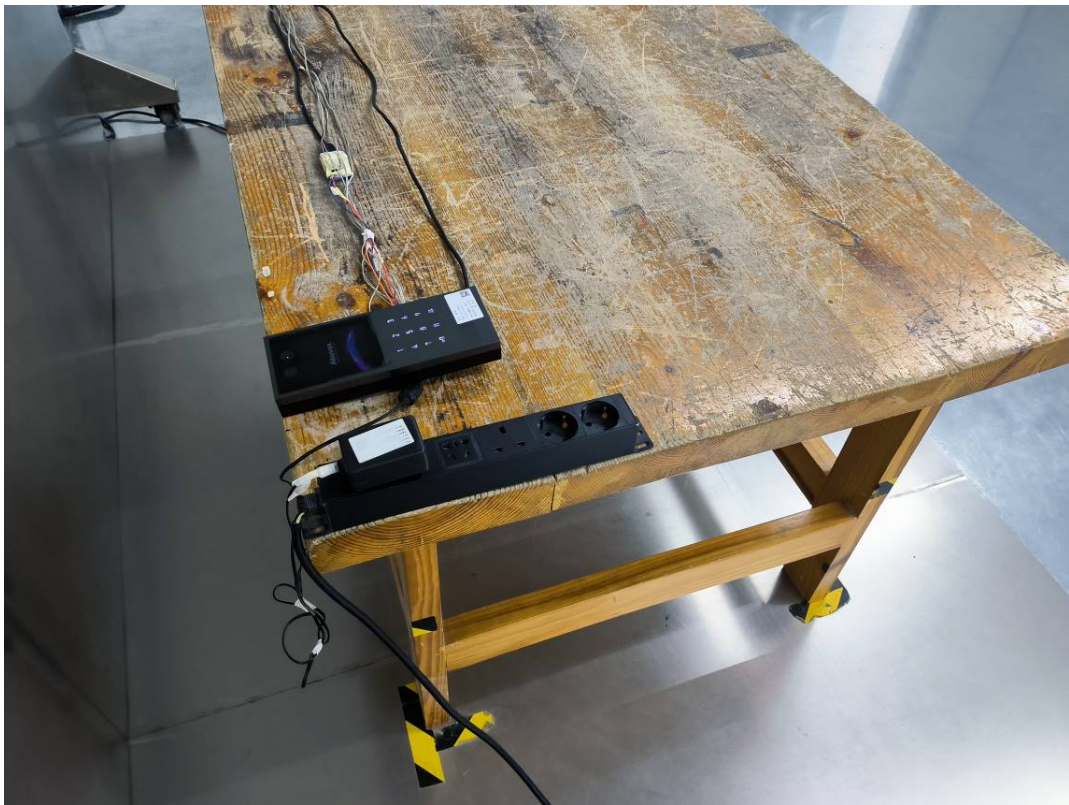
Conducted Emissions Side View-Adapter Power Mode
