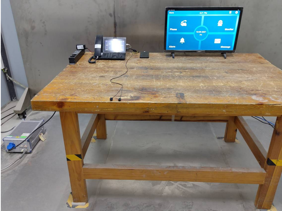
Conducted Emissions Side View - Adapter
