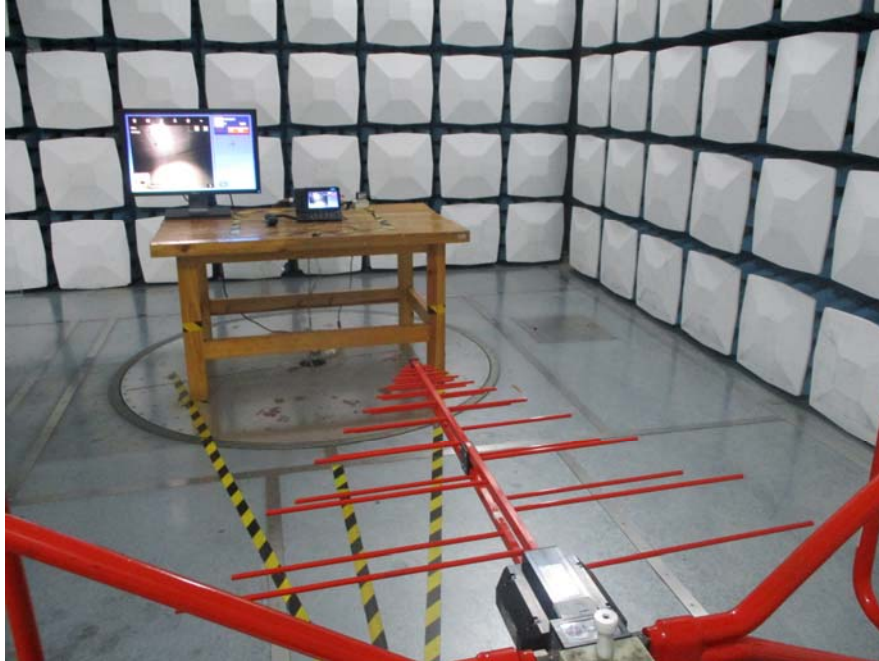
Radiated Emission Below 1GHz View-Adapter
