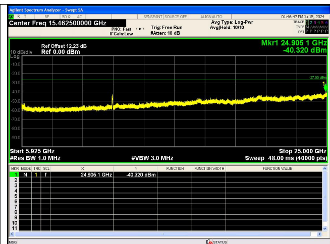
Spurious Emission:5925~25000.0 MHz IEEE 802.11n_Channel 159_40MHz_Antenna 0
