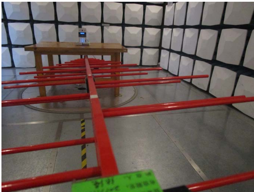
Radiated Emission View (30 MHz ~1 GHz)
