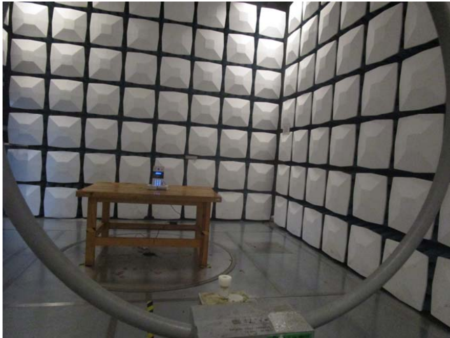
Radiated Emission View (9 kHz~30 MHz)
