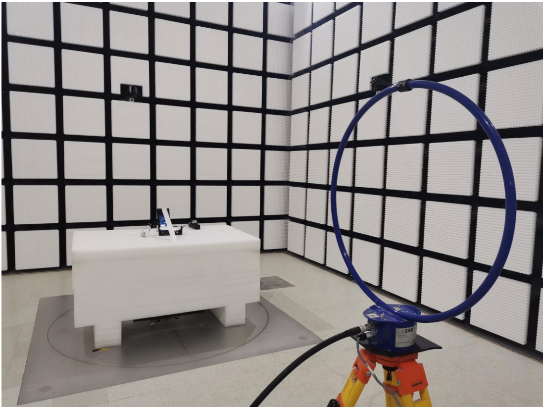
Radiated Emission 9kHz-30MHz Perpendicular View Adapter
