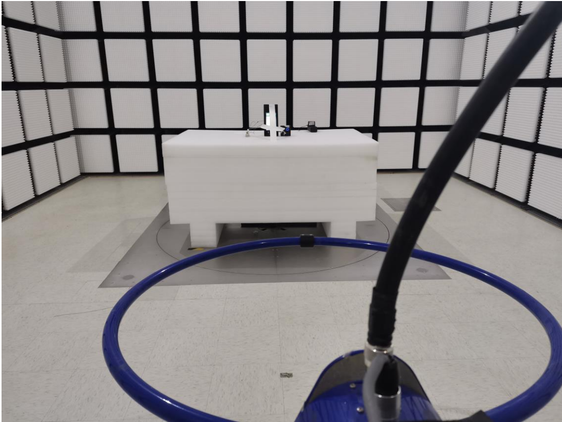
Radiated Emission 30MHz-1GHz View
