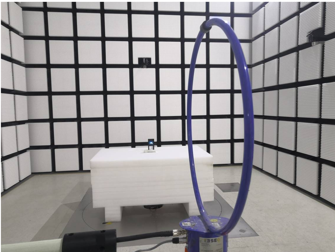
Radiated Emission 9kHz- 30MHz Perpendicular View POE
