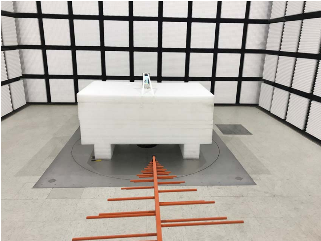
Radiated Emission 30MHz- 1GHz View POE
