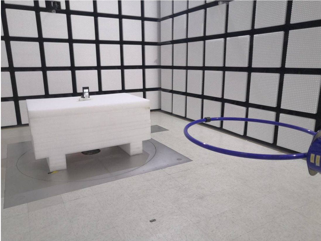
Radiated Emission 30MHz- 1GHz View POE
