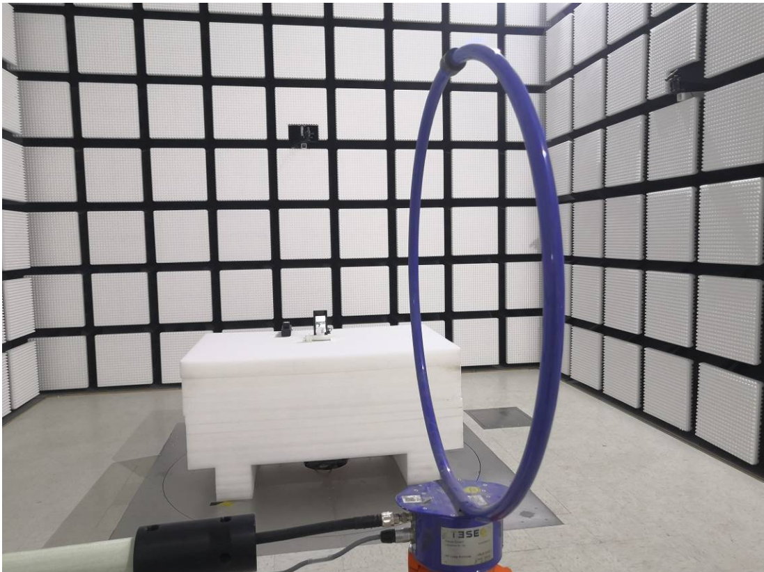
Radiated Emission 9kHz- 30MHz Perpendicular View Adapter
