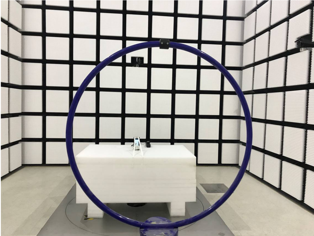
Radiated Emission 9kHz- 30MHz Perpendicular View Adapter
