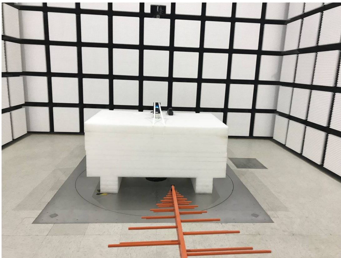
Radiated Emission 30MHz- 1GHz View Adapter
