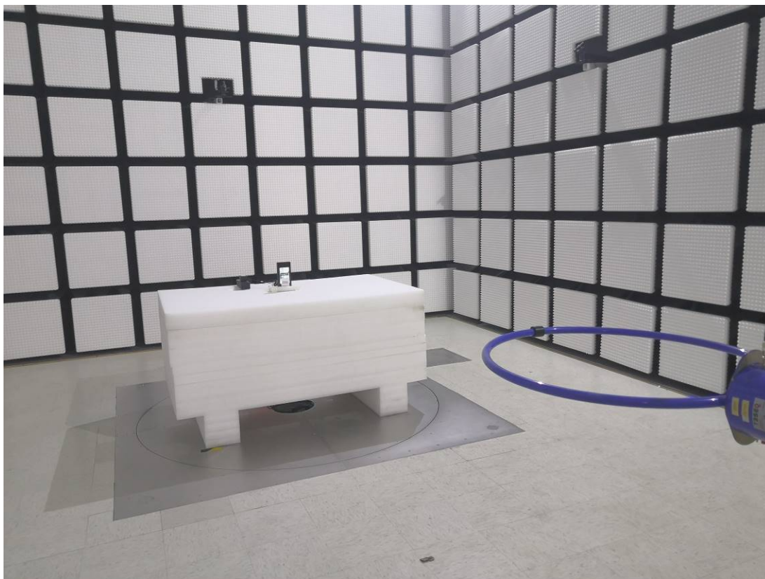
Radiated Emission 30MHz- 1GHz View Adapter
