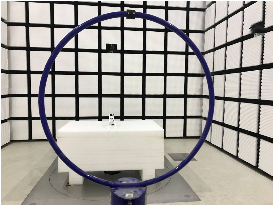
Radiated Emission 9kHz- 30MHz Perpendicular View POE
