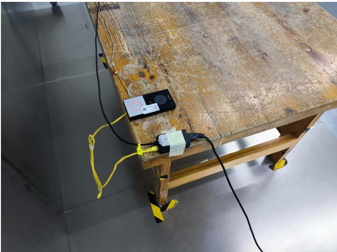
Conducted Emissions Side View-PoE Power
