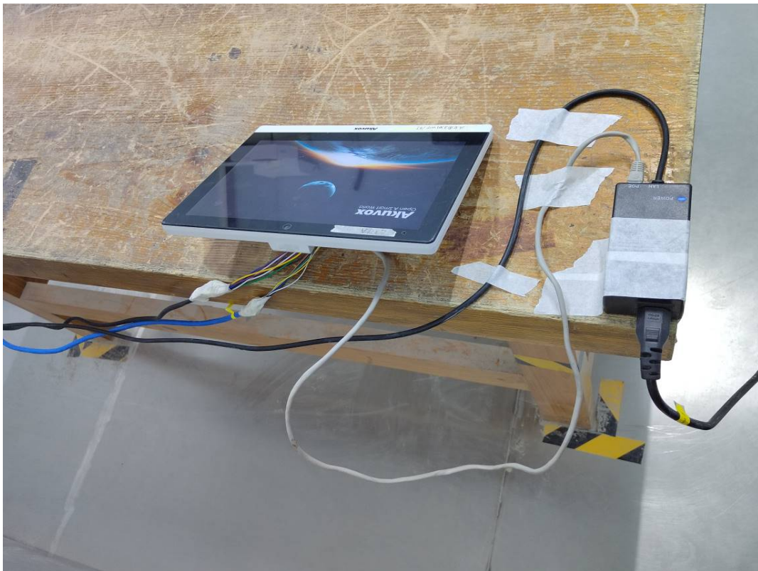
Conducted Emissions Side View- POE
