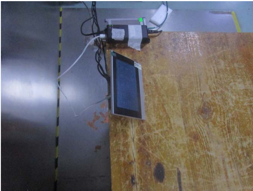
POE Conducted Emissions – Side View
