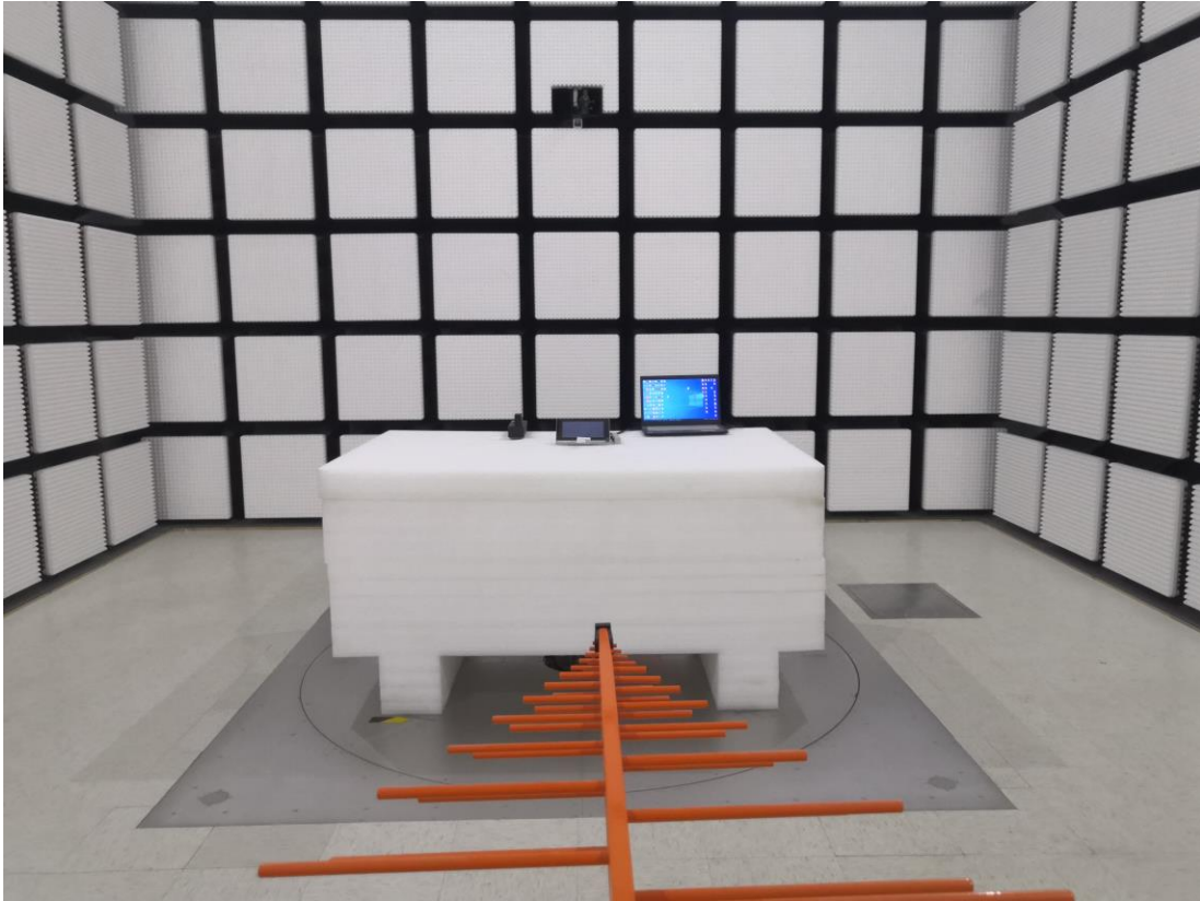
Radiated Emission Below 1GHz View POE
