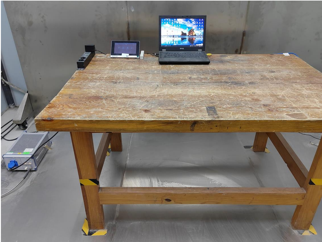
Conducted Emissions Side View
