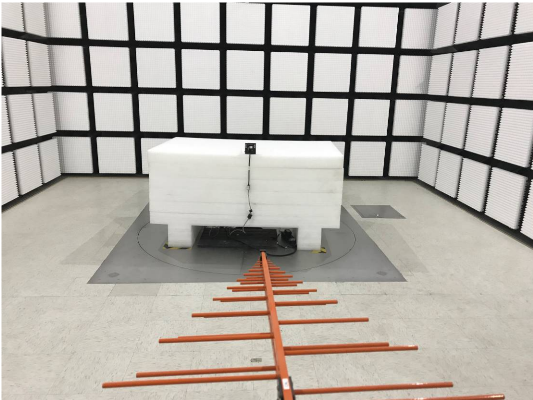
Radiated Emissions Below 1G rear View –POE
