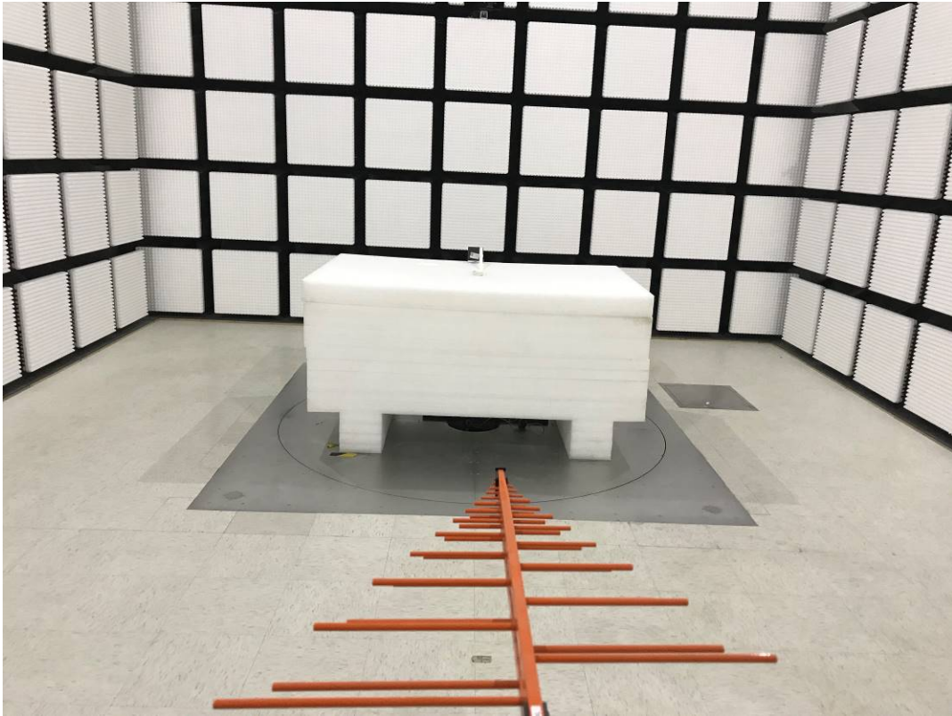
Radiated Emissions Below 1G rear View –POE
