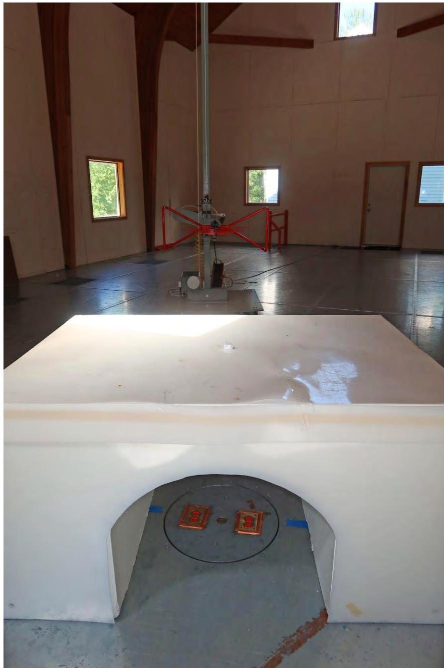
**8. Test Setup Photographs****8.4. Radiated Emissions above 1 to 18 GHz – Front**
