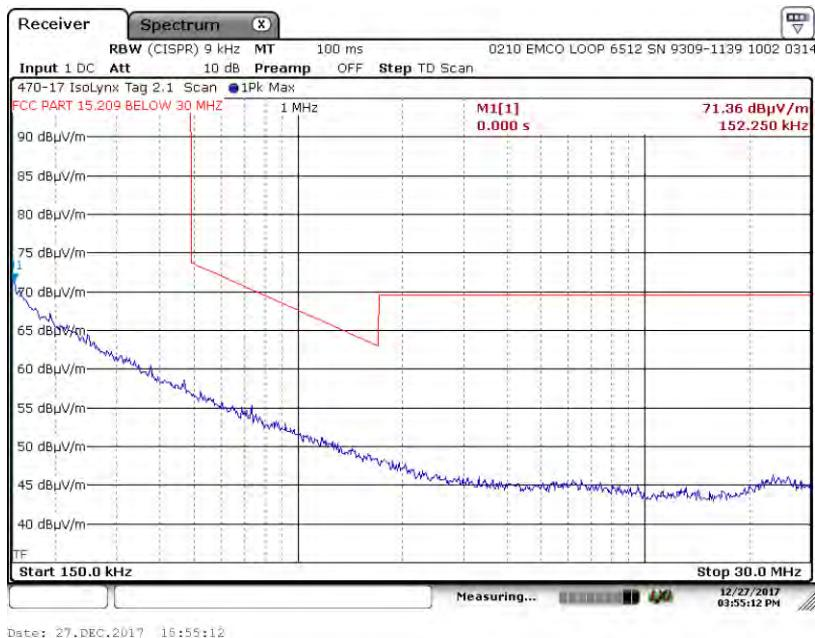
**A2.1.2. Measurement Results: X-Axis, Perpendicular Antenna**
