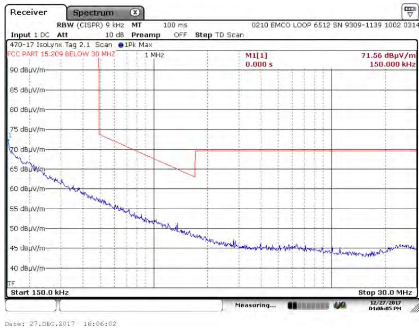
**A2.2.2. Measurement Results: X-Axis, Perpendicular Antenna**
