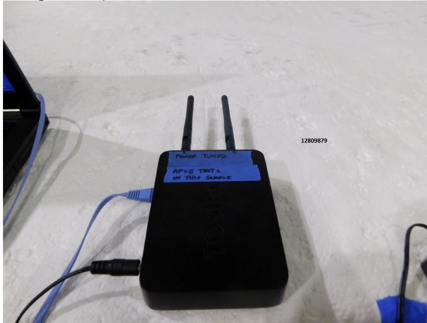
RADIATED SPURIOUS PHOTO (X Orientation, Antenna Configuration 3)
