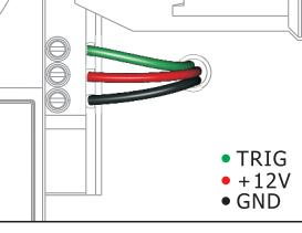
This device does **NOT** require batteries when powered from a 12 Volt alarm panel because the customer's alarm panel will have complete control over the pepper spray dispenser device.
