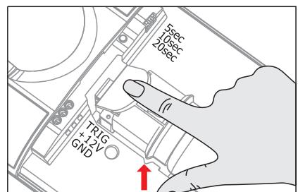
With the back side of the **SAFETY CAP** in the up position, **CAREFULLY** place the ridge part of the canister head into the groove (as shown with the **RED** arrow in picture) and push the canister in.
