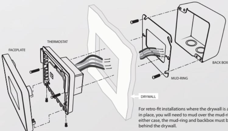
For retro-fit installations where the drywall is already in place, you will need to mud over the mud-ring. In either case, the mud-ring and backbox must be installed behind the drywall.
