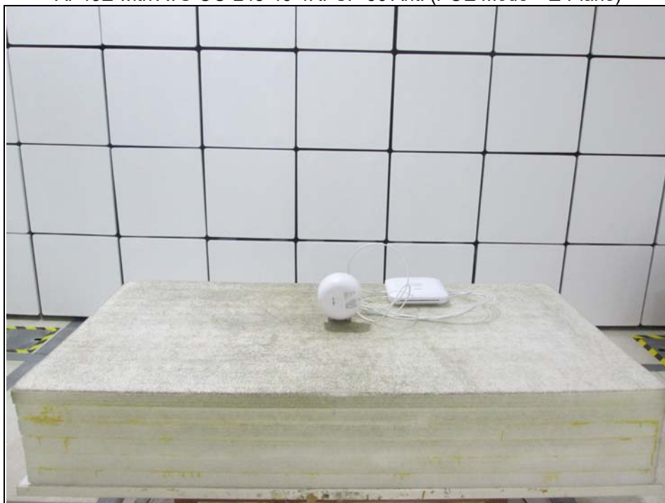
Radiated Emission Test (Below 1GHz) AP43E with ATS-OO-245-46-4RPSP-36 Ant. (POE Mode – Z-Plane)
