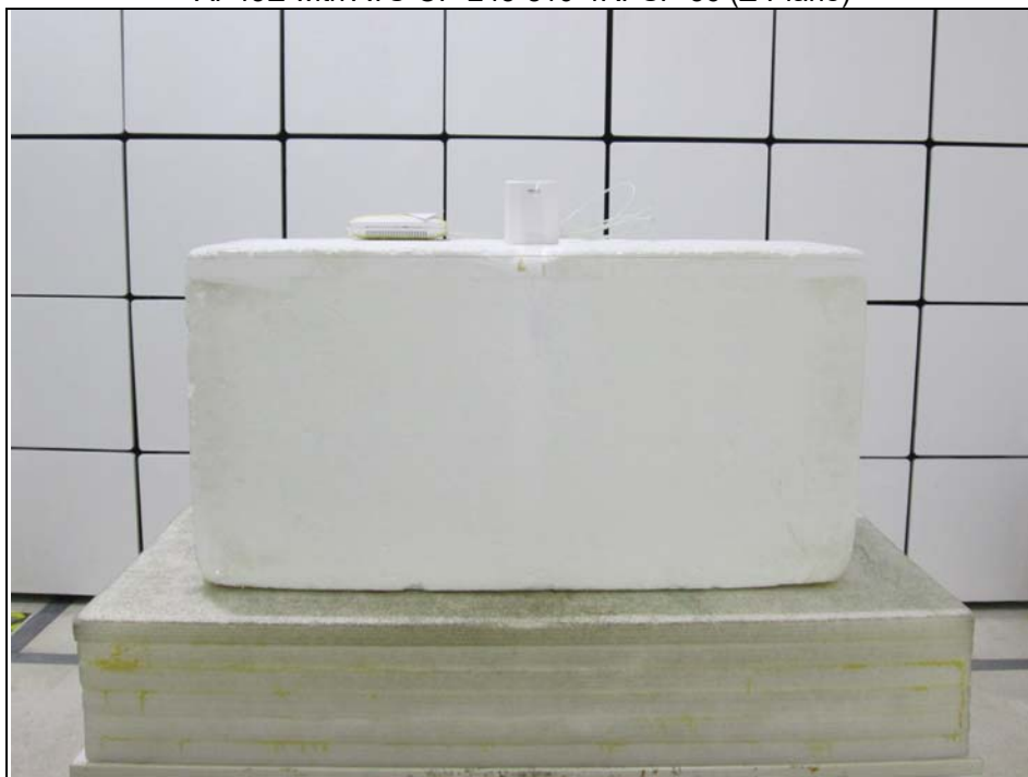
Radiated Emission Test (Above 1GHz) AP43E with ATS-OP-245-810-4RPSP-36 (Z-Plane)
