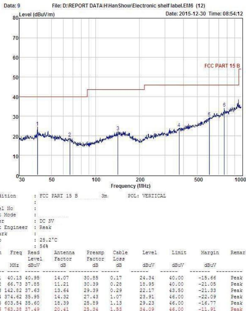
Remark: Level = Read Level + Antenna Factor - Preamp Factor + Cable Loss
