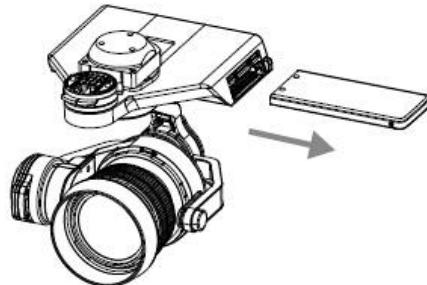
2. Insert the X5R SSD into the X5R READER correctly, then connect the X5R READER to a device with DJI CineLight installed via the USB 3.0 cable. Video can be exported by the DJI CineLight. Refer to the Zenmuse X5R user manual for more DJI CineLight details.
