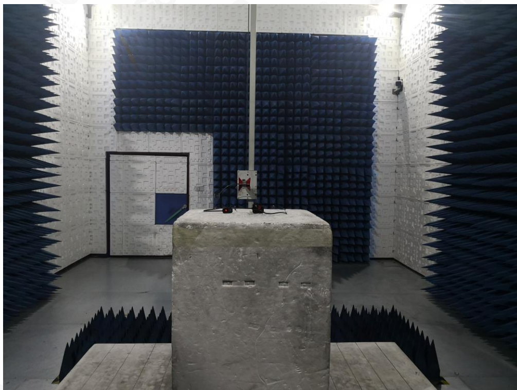
RADIATED EMISSION TEST SETUP ABOVE 1GHZ
