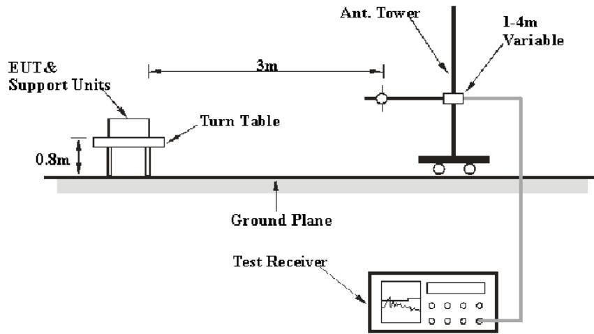
The radiated emission tests were performed in the 3-meter chamber test site, using the setup accordance with the ANSI C63.10-2020. The specification used was the FCC Part Subpart C limits.
