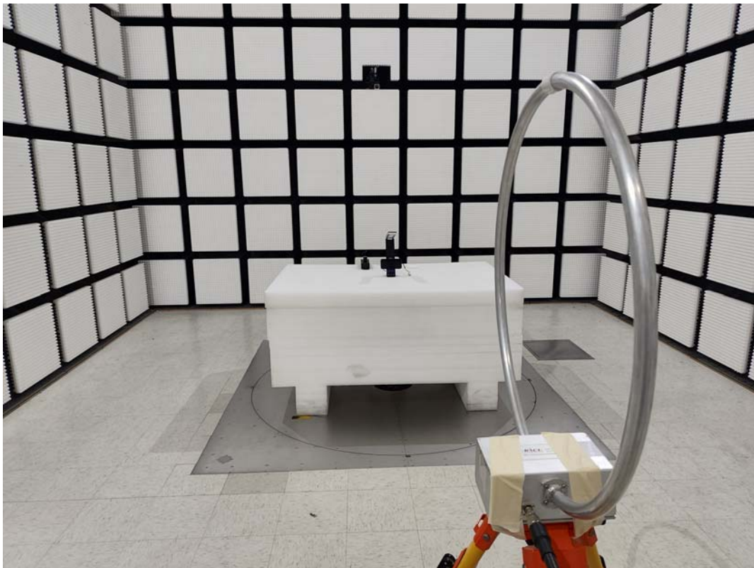
Radiated Emission 9k-30MHz Perpendicular View M4
