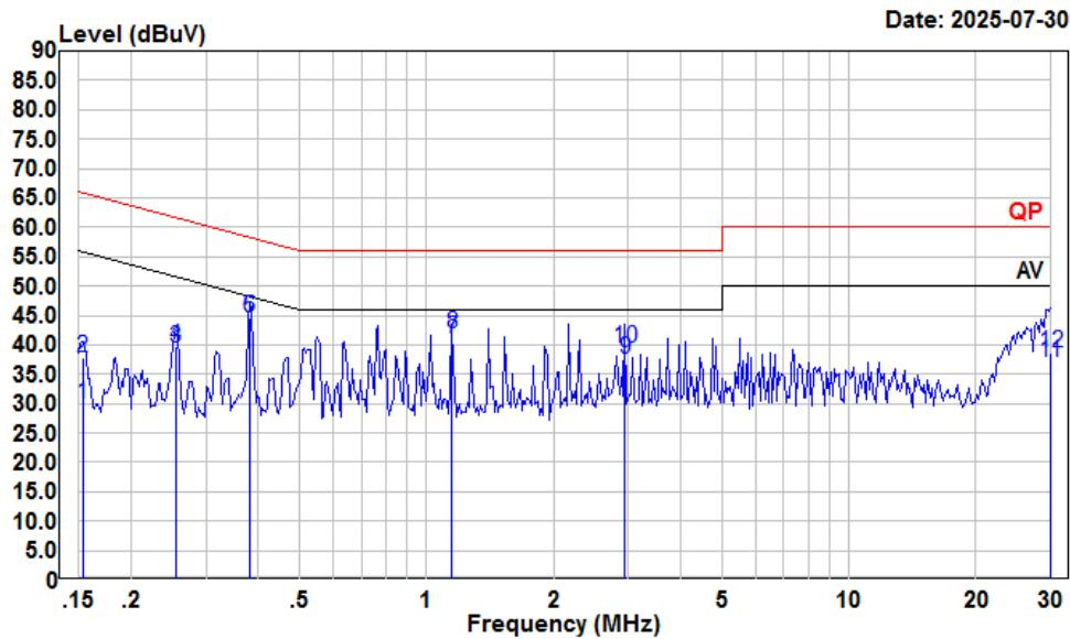
**Condition: Neutral****Project : 2501V27392E-RF****test Mode: Transmitting****tester : Alex Yan Setting:RBW:9kHz**
